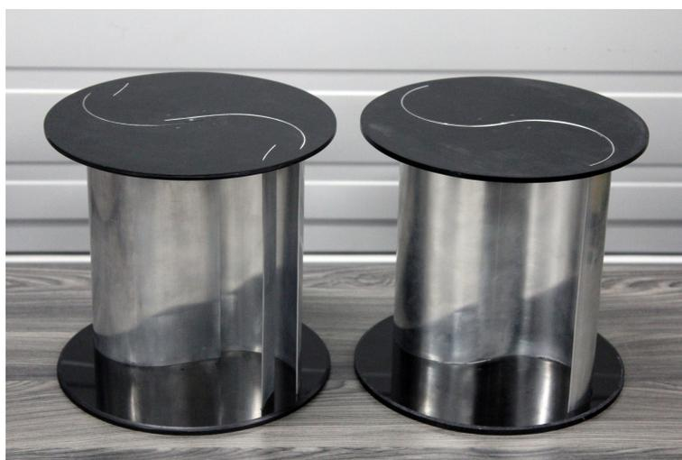
**Figure 8.** Test rotors of the conventional semicircular profile (right) and multi-blade Bach (left) (the secondary blades were installed on the split Bach profile rotor model).
