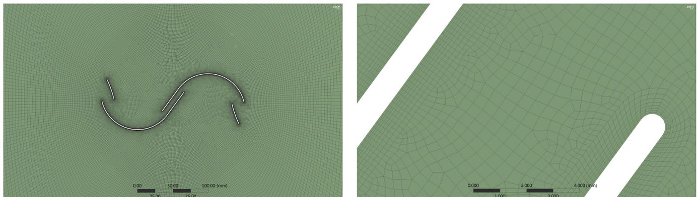
**Figure 5.** General structure of the mesh (left) and details of the mesh near the profile walls (right).
