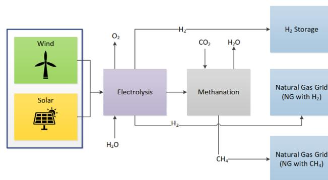
**Figure 2.** The green hydrogen schematic.
