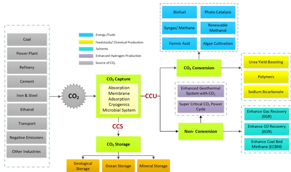
**Figure 3.** The CCUS schematic diagram.
