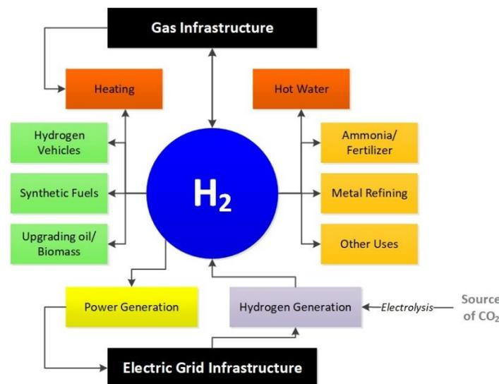
**Figure 5.** The hydrogen utilization options.
