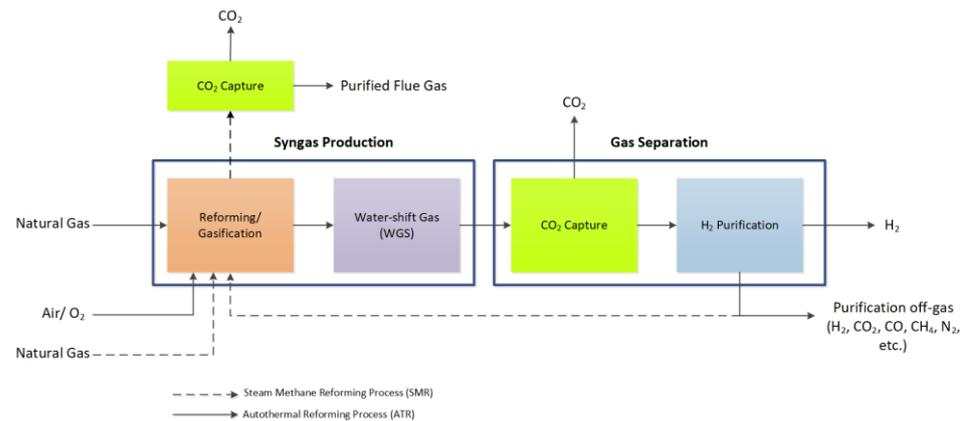
**Figure 1.** The blue hydrogen process flow: SMR and ATR.
