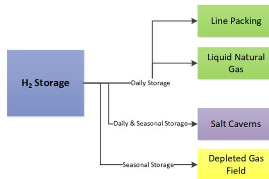
**Figure 4.** The hydrogen storage alternatives.
