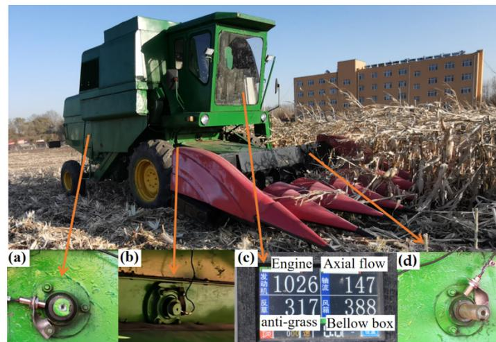
**Figure 2.** Harvester speed detection: (a) detection of the re-detachment speed; (b) upper kernel speed; (c) speed indicator; (d) detection of cylinder speed.
