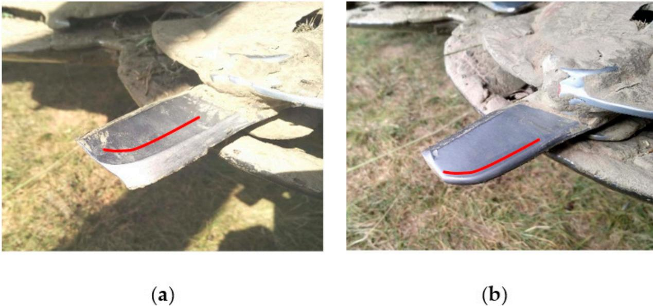
**Figure 14.** Macro-morphology of the two blades after working on the harvester for 43 h of operation: (a) knife with 1600 W laser cladding; (b) 65 Mn cutting tools available on the market.
