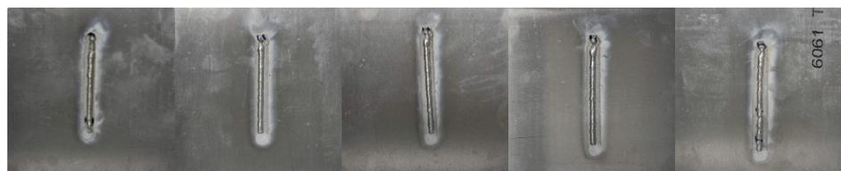
**Figure 3.** Specimens of WAAM with different heat input.
