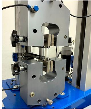
**Figure 6.** Tensile test—device with 3D printed LT clear bar (specimen) placed upon it.
