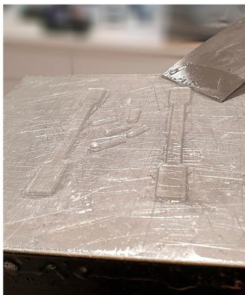
**Figure 4.** Three-dimensional printed samples of bars (specimens) for determination of the mechanical properties of Dental LT ClearResin. Specimens were printed directly on printing plate without any supports and then carefully removed and post-processed.
