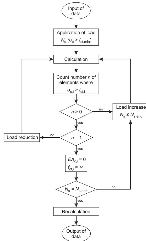
Figure 12. Iterative calculation procedure for the CPM.
