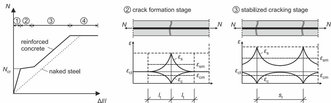
**Figure 1.** Stages of crack propagation in reinforced concrete specimens in uniaxial tensile tests.
