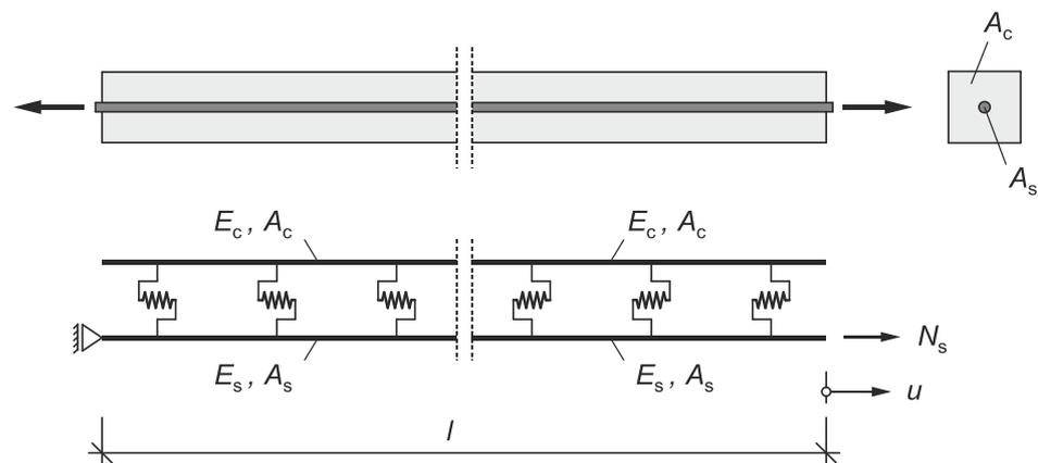
Figure 2. Crack propagation model (CPM).
