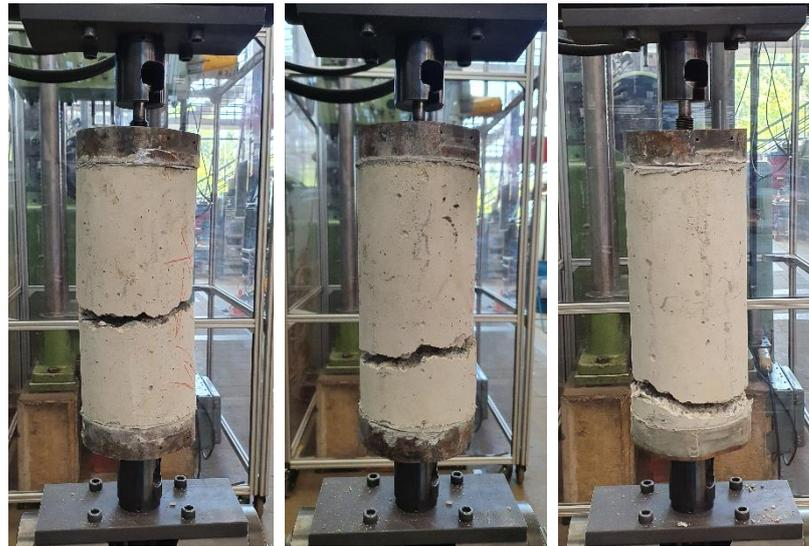
Figure 4. Direct tensile tests (cylinder  $\text{Ø}150 \times 300$  mm, C30/37,  $d_g = 16$  mm).
