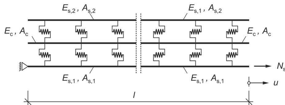
**Figure 11.** Extension of the CPM to a three-bar model.
