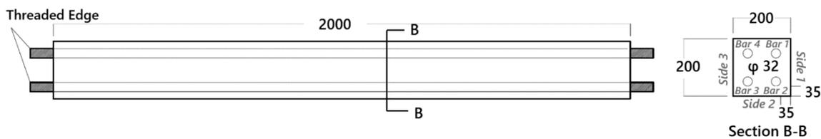
Figure 14. Details of the axial tensile specimen (dimensions shown in mm) [36].
