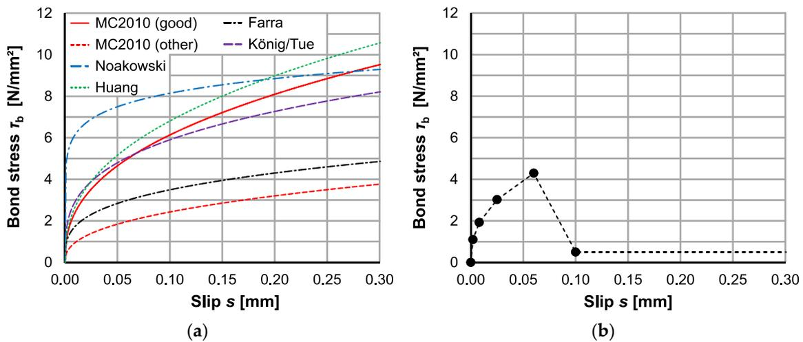
**Figure 10.** Bond laws: (a) according to Equation (14) and Table 1; (b) user-defined.
