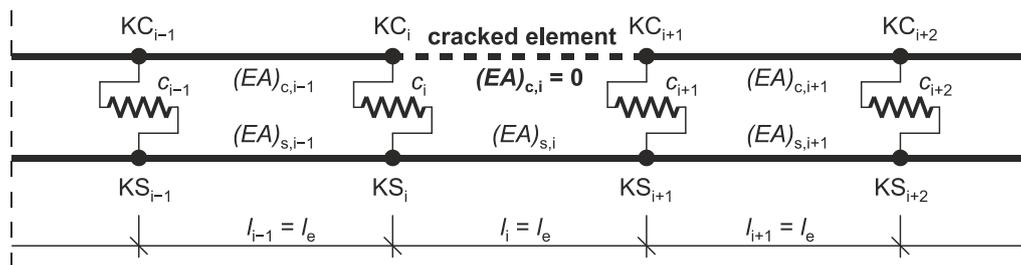
Figure 3. Cracked element in the CPM.
