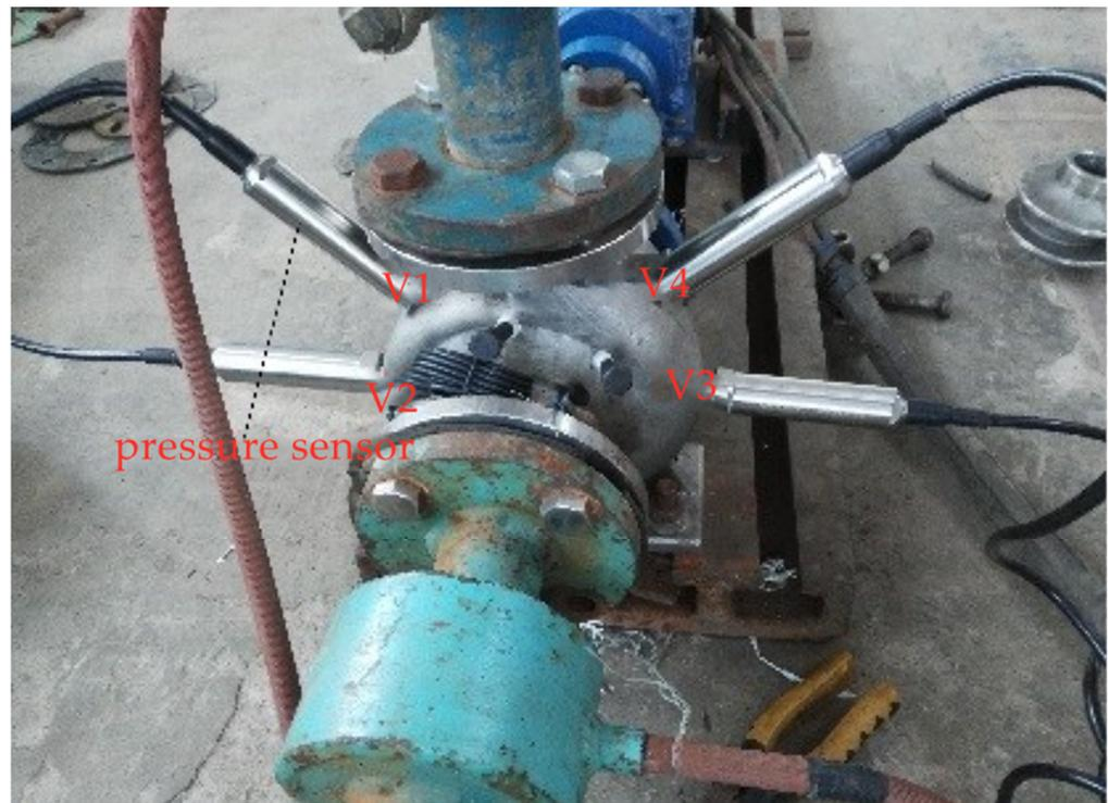
Figure 4. Pressure sensors distribution.
