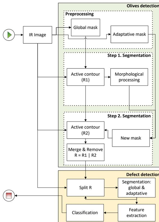
**Figure 3.** Image processing block diagram.
