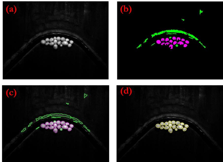
**Figure 7.** Example of olives segmentation (conveyor belt not completely full). (a) Image acquisition. (b) Result of the preprocessing step: global thresholding mask in magenta and adaptive thresholding mask in green. (c) Level one (magenta) and level two (green) segmentation. (d) Final segmentation result.
