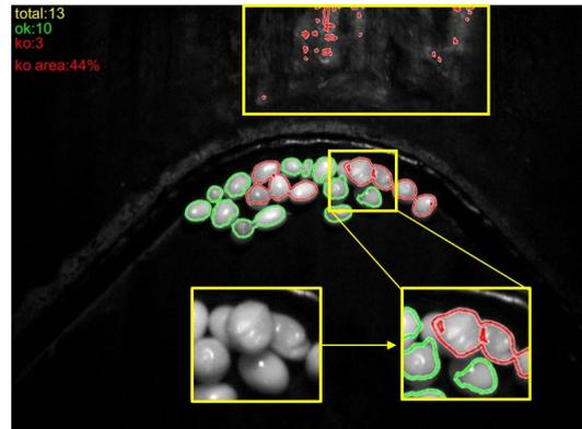
**Figure 11.** Example of false positives in an image with a low number of olives or set of olives regions. The top shows false positives because of the conveyor belt glows. The bottom shows false positives originating by the overlap of olives.
