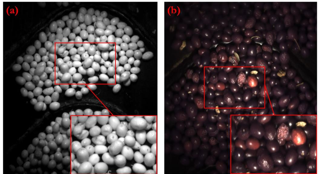
**Figure 2.** Images acquired on the conveyor after the cleaning process. (a) Infrared camera (Nano M2590-NIR). (b) Visible band camera (Nano C242).
