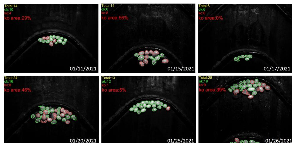
**Figure 12.** Example of defect detection for images labelled as low acquired during the period of evaluation.
