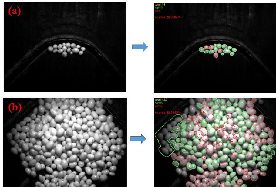
**Figure 9.** Defect detection. (a) Figure 7 defective olives detection. (b) Figure 8 defective olives detection.
