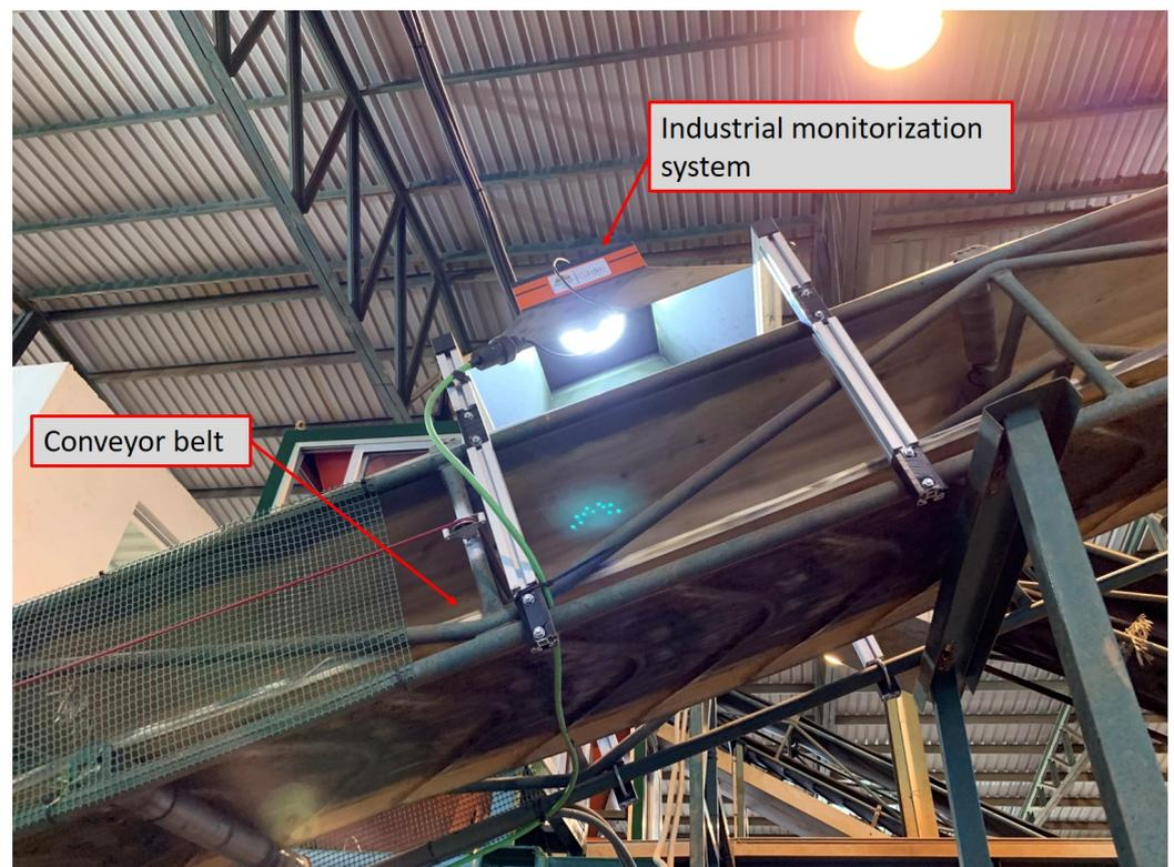
**Figure 1.** Industrial monitorization system installed on the conveyor belt after the olive cleaning process.
