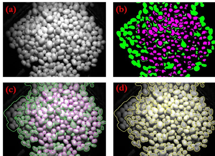
**Figure 8.** Example of olive segmentation (conveyor belt completely full). (a) Image acquisition. (b) Result of the preprocessing step: global thresholding mask in magenta and adaptive thresholding mask in green. (c) Level one (magenta) and level two (green) segmentation. (d) Final segmentation result.
