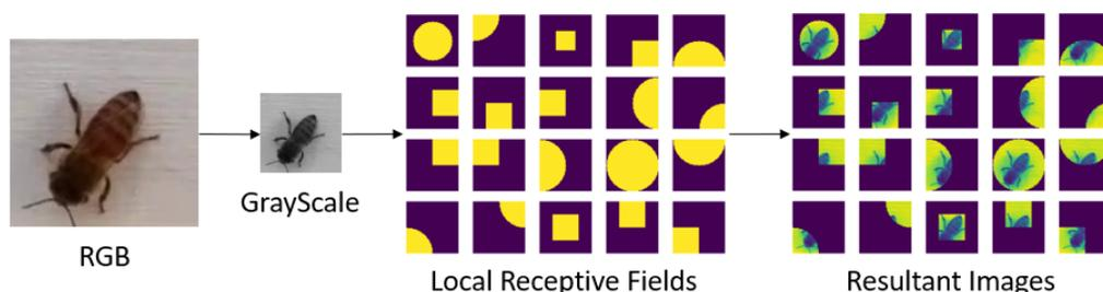
Figure 1. LRF construction: (1) RGB image is grayscaled; (2) 20 LRFs are overlapped with grayscale image.
