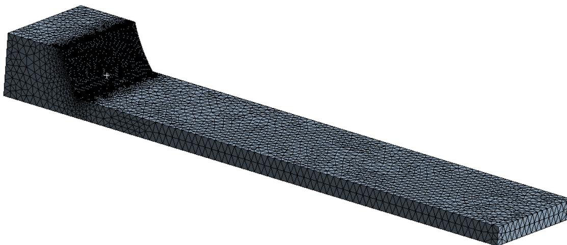
**Figure 5.** Finite element model of fluid domain in middle gate chamber and corresponding middle gate section.
