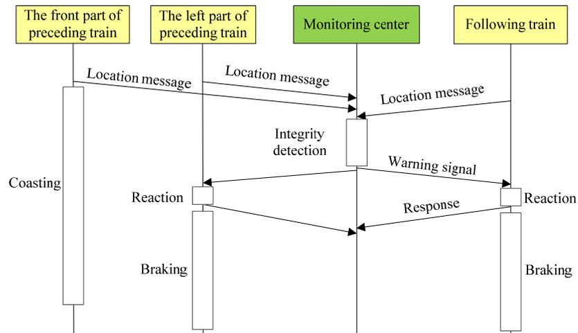
Figure 2. Timeline diagram of a train integrity detection under potential collision risk.
