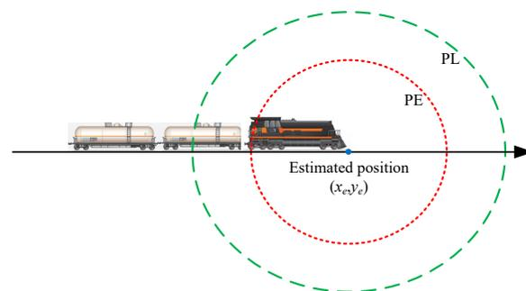
Figure 3. PE and PL in the GNSS-based train positioning.
