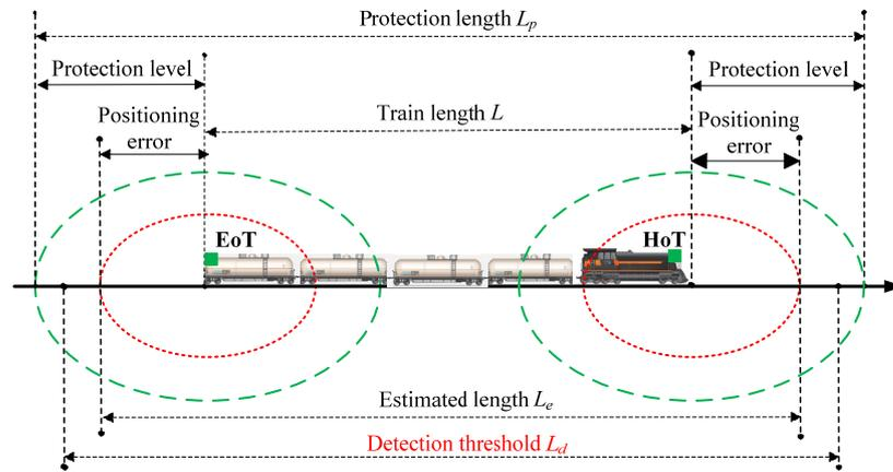
Figure 5. The distributed structure of the train integrity detection.
