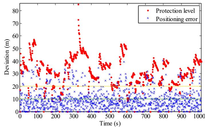
Figure 13. Simulated positioning error and protection level.
