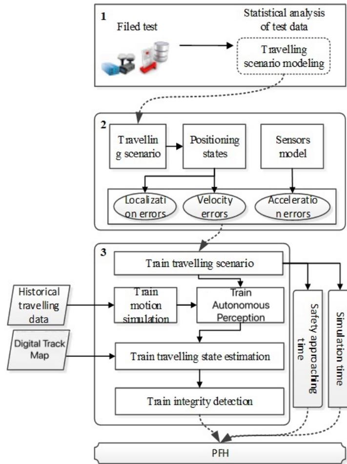
Figure 7. Verification procedure based on the analysis of experiments data.
