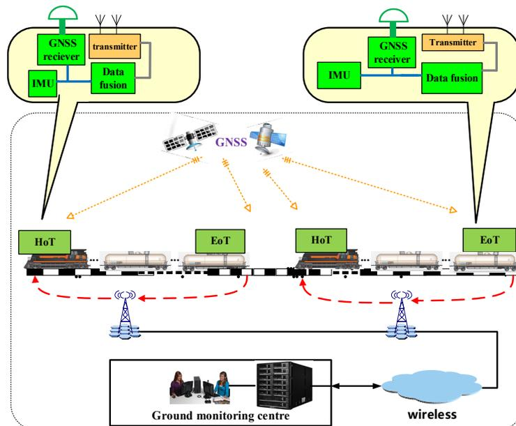
**Figure 1.** Structure of a typical GNSS-based TIMS.
