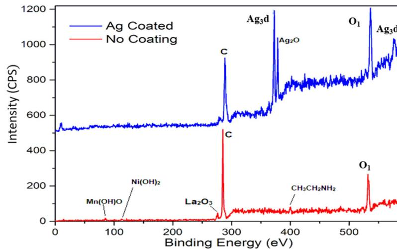
Figure 10. XPS full surface scan of the Ag-coated and virgin pellets.
