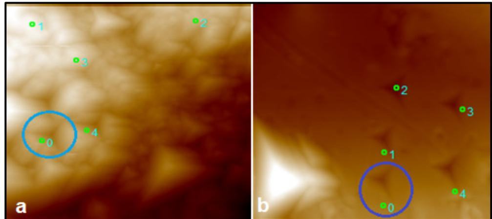
**Figure 12.** Micrograph of the nano-indentation on the surface of (a) virgin and (b) Ag-coated pellets.
