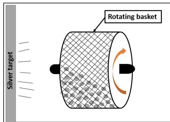
**Figure 3.** Schematic representation of the rotating basket, containing the Arboblend V2 Nature pellets and the silver target.
