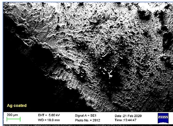
**Figure 8.** SEM surface morphology image of Ag-coated pellet showing a reasonably rough but well-coated surface without pinholes.
