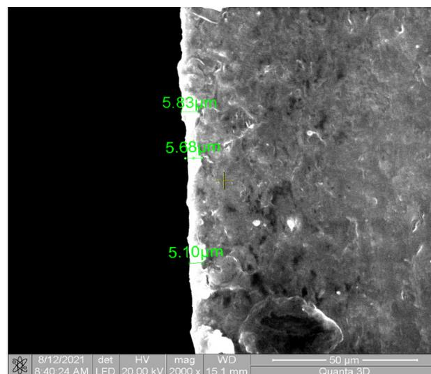
**Figure 9.** SEM of cross-sectioned granule of Ag-coated pellet.
