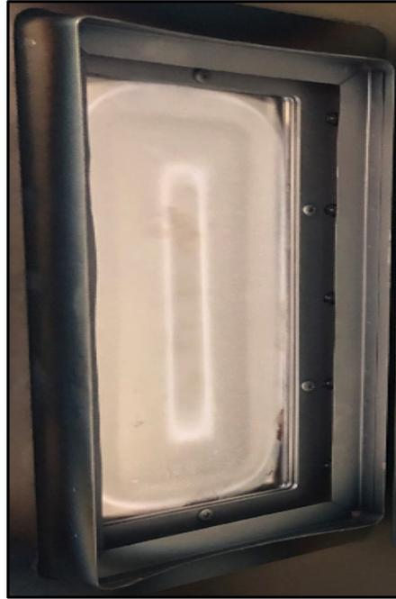
**Figure 2.** The silver target used for sputtering deposition.
