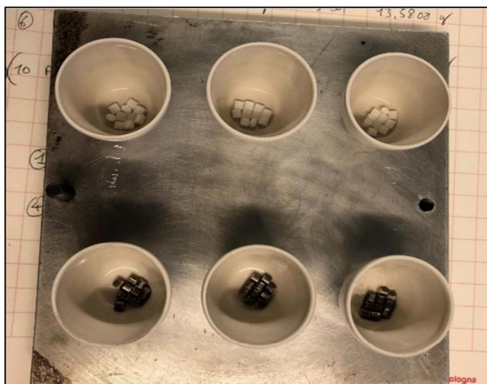
Figure 4. The samples of Arboblend V2 Nature before being inserted in the furnace.
