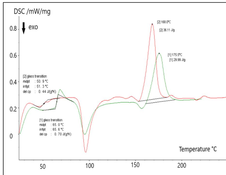
Figure 7. DSC test for silver nano-coated Arboblend V2 sample.
