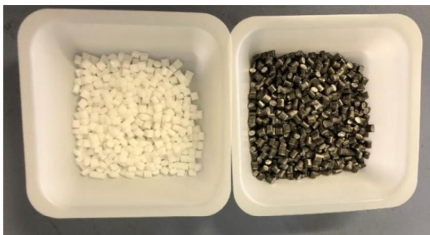
**Figure 1.** The Arboblend V2 Nature pellets: (left) virgin and, (right) silver-coated pellets.
