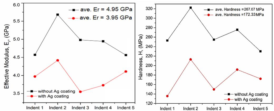
Figure 14. The effective modules and hardness extracted from indentation measurements.
