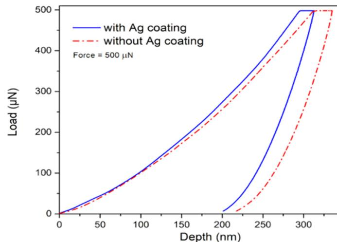
**Figure 13.** Force vs. displacement depth profiles for the virgin and Ag-coated pellets under force of 500  $\mu\text{N}$  for 5 seconds.
