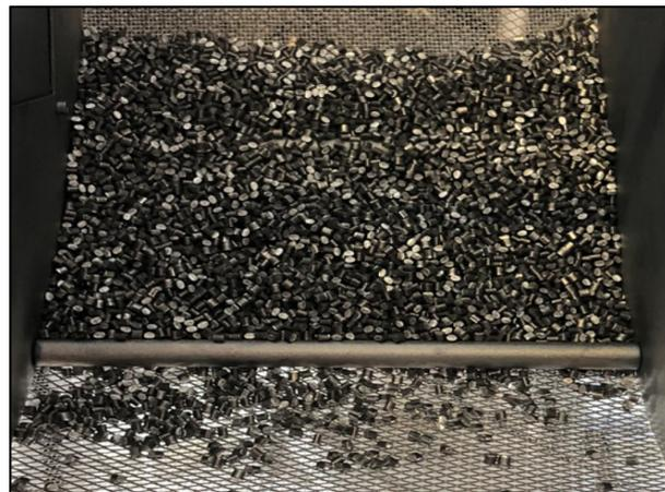
**Figure 5.** The first cycle of PVD coating of the Arboblend V2 Nature pellets with silver nanoparticles.
