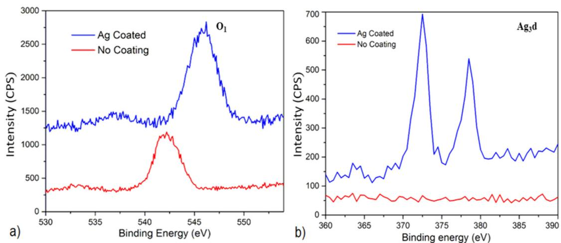
Figure 11. XPS spectrum for (a) oxygen and (b) silver, on surface of Ag-coated and virgin pellets.
