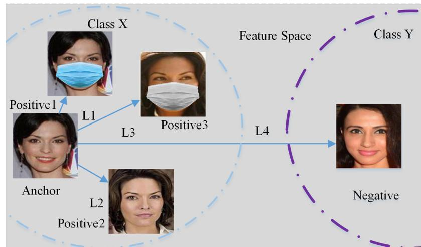
**Figure 2.** A representation of triplets in feature space. Anchor, Positive1, Positive2, and Positive3 belong to class X; Negative belongs to class Y; L represents the feature distance between different samples.
