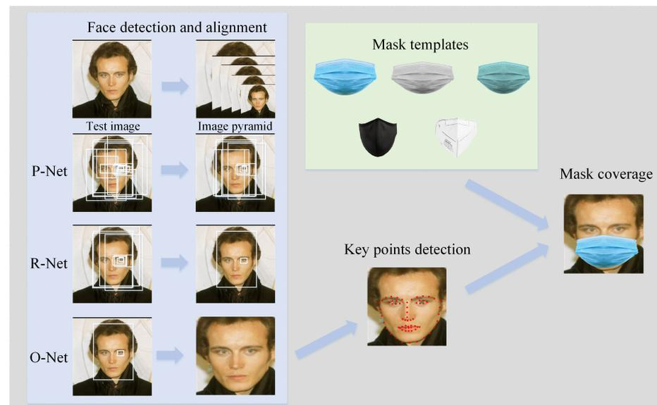
**Figure 1.** The process of masked-face image generation. First, the face in the test image is detected and aligned; then, the information about the chin and the bridge of the nose is output; finally, the mask templates are used to cover the face to generate the masked-face image.
