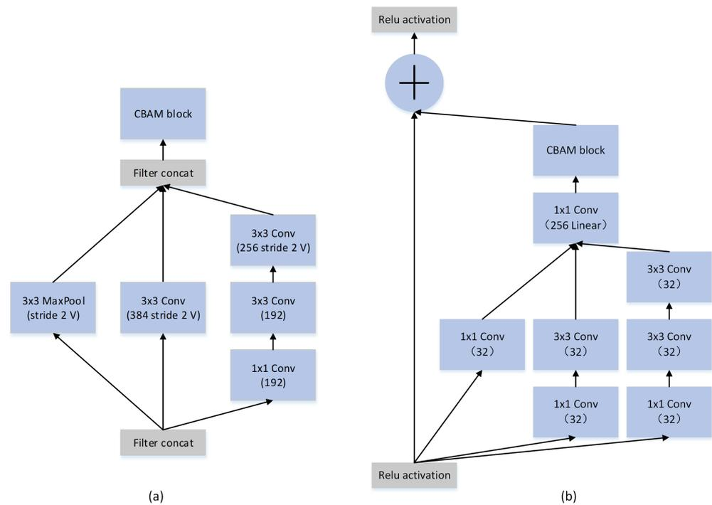
**Figure 10.** (a) Reduction-A module with the attention mechanism; (b) Inception-ResNet-A module with the attention mechanism.
