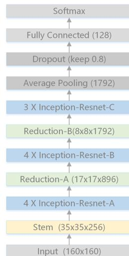
Figure 6. Inception-ResNet-v1 network structure diagram.
