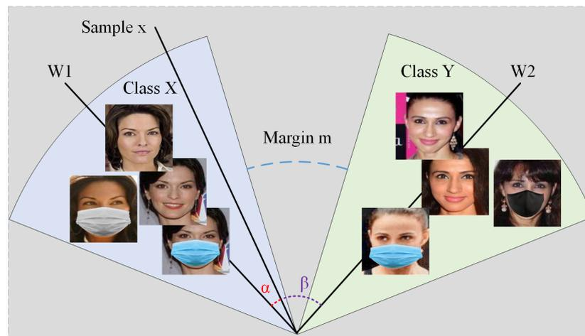
**Figure 3.** A representation of Cosface in feature space.  $\alpha$  represents the angle between  $x$  and  $W1$ ;  $\beta$  represents the angle between  $x$  and  $W2$ ;  $m$  is the margin of the angle. The cosine angle and margin effectively limit the inter-class difference while further compressing the intra-class distance.
