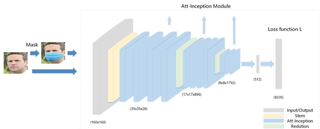
**Figure 7.** MFCosface network structure diagram. The color of the module corresponds to the structure in Figure 6. After the face is covered with a mask, through the detection of the key facial features we proposed, the image is sent to a model composed of Att-inception modules that incorporate the attention mechanism. Training the model through large margin cosine loss  $L$  can increase the intra-class differences while reducing the inter-class differences.
