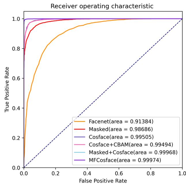
**Figure 9.** The receiver operating characteristic curve. Facenet represents the original network, masked represents the use of images generated by our method for training, Cosface represents the use of large margin cosine loss as the loss function, CBAM means training with an attention mechanism, and MFCosface represents the method we proposed.
