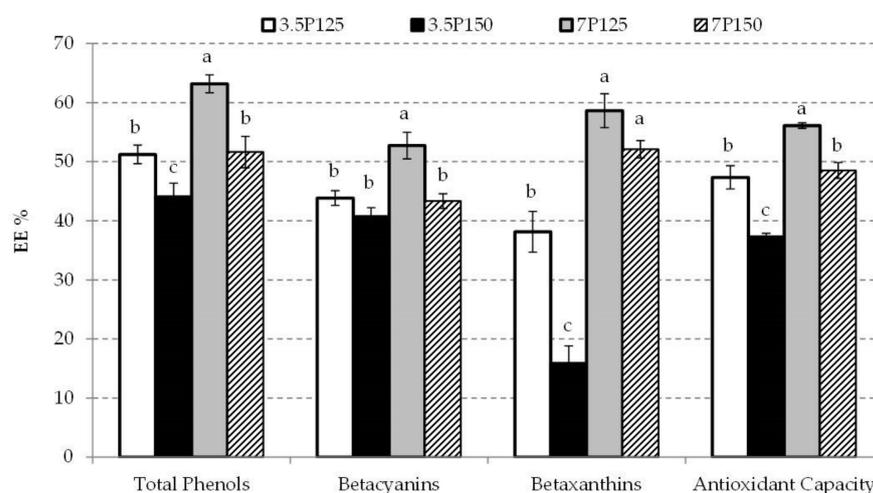
**Figure 4.** Mean values and standard deviation of encapsulation efficiencies percentage in beetroot spray-dried samples for analyzed bioactive compounds. Letters indicate homogeneous groups established by the ANOVA ( $p < 0.05$ ) for each bioactive compound or antioxidant capacity: 3.5P125 or 3.5P150, powder with 3.5% of pea protein concentration spray dried at 125 or 150 °C, respectively; 7P125 or 7P150 powder with 7% of pea protein concentration spray dried at 125 or 150 °C, respectively.
