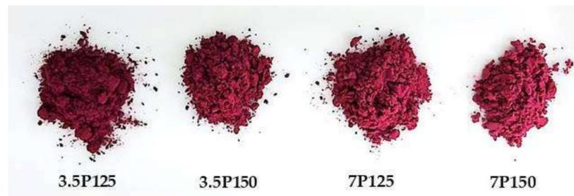
**Figure 2.** Appearance of studied beetroot powder samples: 3.5P125 or 3.5P150, powder with 3.5% of pea protein concentration spray dried at 125 or 150 °C, respectively; 7P125 or 7P150 powder with 7% of pea protein concentration spray dried at 125 or 150 °C, respectively.
