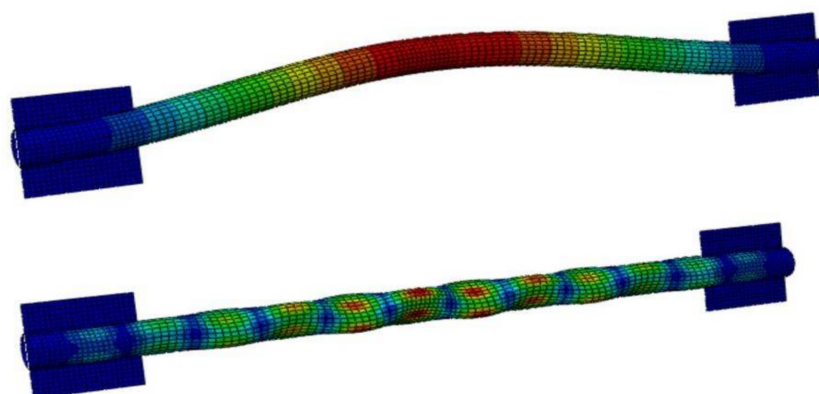
Figure 6. Effects of geometric imperfections in circular braces: global buckling mode (amplitude = L/1500 ); local buckling mode (amplitude = t/100 ).
