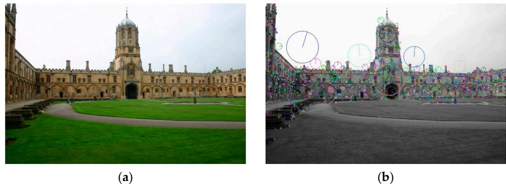
**Figure 1.** SIFT key point detection. (a) is the input image [37]. and (b) is the key point description image, which is represented by a small circle at the function position, and the direction of the feature points will be displayed inside the circle. (Source: The Oxford Buildings Dataset).
