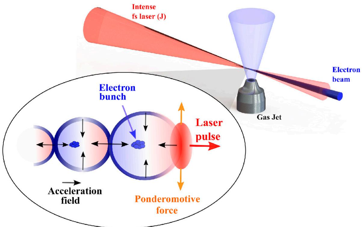
Figure 1. Schematic of LWFA process.
