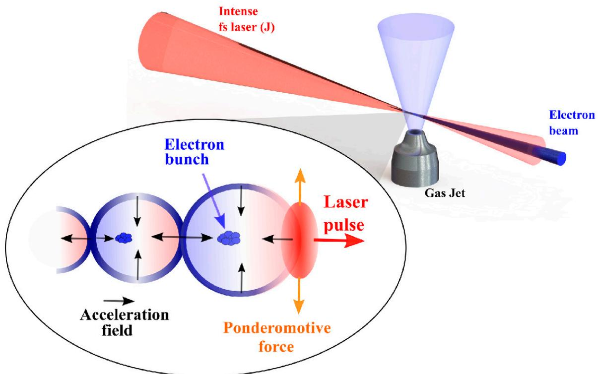
Figure 1. Schematic of LWFA process.
