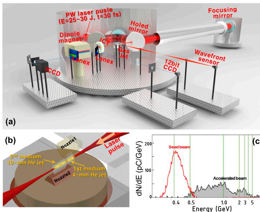
**Figure 2.** (a) Experimental layout for dual-stage LWFA with a PW laser pulse, (b) schematic drawing of the dual-stage target, and (c) the experimental result with the dual-stage target [18]. In figure (c), the red line shows the electron spectrum from the first target, and the black line shows the spectrum after the second target.
