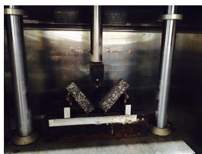
Figure 4. Three-point bending test of recycled asphalt mixture.
