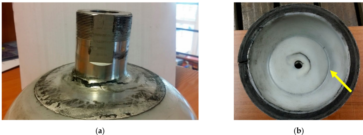
Figure 5. View of a damaged boss after fatigue testing. (a) Crack in the metallic boss and (b) crack in the inner side of the liner's dome.
