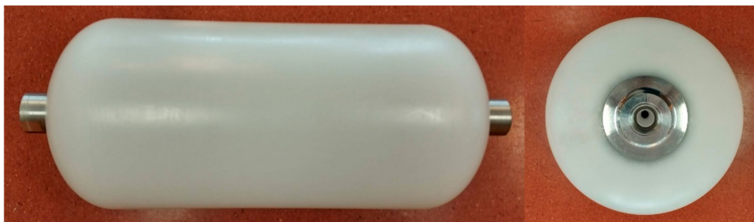
Figure 2. View of the exemplary HDPE liner for a hydrogen vessel, manufactured using rotomolding technology.
