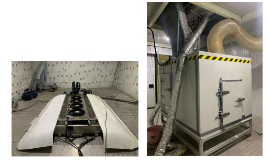
Figure 2. Photos of the transcritical CO<sub>2</sub> electric bus air conditioning system rig.
