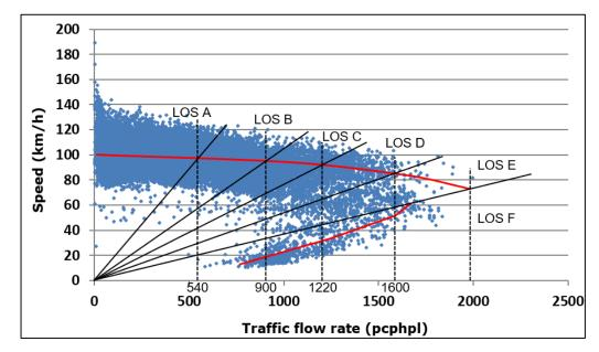
Figure 3. Traffic flow rate (veh/h)–speed curve (km/h).
