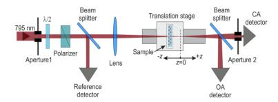
Figure 4. Sketch of the z-scan experimental setup.
