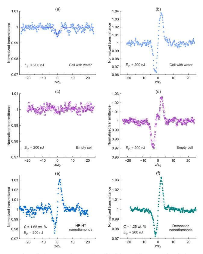
**Figure 5.** The normalized transmittance of the quartz cell with (a) distilled water and (c) an empty cell obtained in the openaperture z-scan. The ratio of the nonlinear transmittance obtained in the closed to the data obtained in the open-aperture z-scan for the quartz cell (b) with distilled water, (e) with HP-HT nanodiamond suspension, (f) with detonation nanodiamond suspension, and (d) an empty cell. The measurements were performed at the incident laser pulse energy of 200 nJ.
