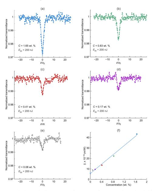
Figure 6. (a–e) Normalized transmittance of suspensions of HP-HT nanodiamonds with different concentrations recorded in the open-aperture z-scan. Dots correspond to the experimental data while solid lines represent the result of the fitting with Equation (2). Figure (f) represents the dependence of the calculated two-photon absorption coefficient  $\beta$  as a function of concentration C.
