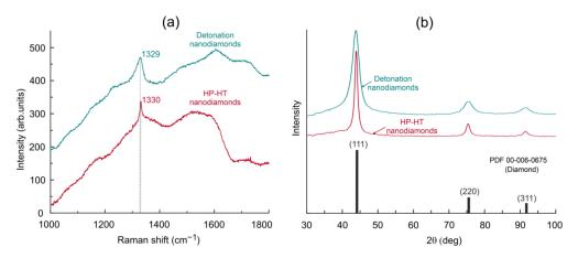
**Figure 2.** (a) Raman spectra of HP-HT and detonation nanodiamonds film and (b) X-ray diffraction patterns of HP-HT and detonation nanodiamond powders. The X-ray diffraction pattern of diamond (Powder Diffraction File 00-006-0675) is presented for a reference.
