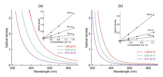
**Figure 3.** The optical density of the (a) HP-HT and (b) detonation nanodiamond suspensions in 1 mm thick quartz cell. Insets show the corresponding optical density as a function of concentration measured at three different wavelengths of 400, 532, and 795 nm.
