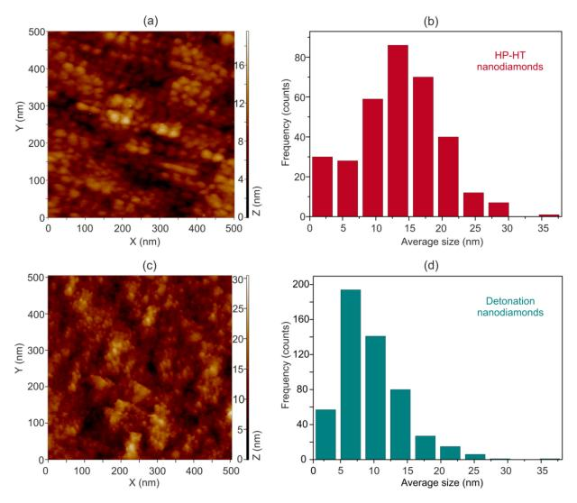
**Figure 1.** Atomic force microscopy images of (a) HP-HT and (c) detonation nanodiamond films. The image processing reveals the HP-HT and detonation nanodiamond particle size distributions shown in figures (b) and (d), correspondingly.
