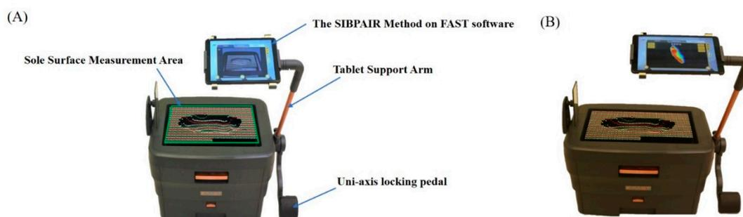
**Figure 1.** The Single-Image-Based Pin-Array Impression Reconstruction (SIBPAIR) method implemented on a commercial 3D foot assessment system (FAST, Enford International Co., Taiwan): (A) measurement of the foot impression, and (B) reconstruction of the 3D sole surface for the subsequent calculation of foot morphological parameters.
