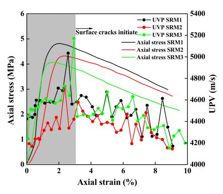
Figure 8. Relationship between the axial stress–strain and UPV.
