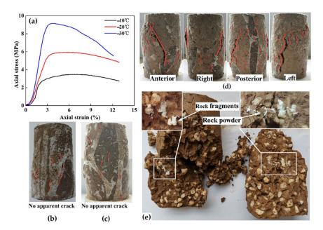
**Figure 5.** Failure patterns of frozen soil–rock mixtures (FSRMs) under uniaxial compression: (a) stress-strain curves; (b) failure pattern of the FSRM at -10 °C; (c) failure pattern of the FSRM at -20 °C; (d) failure pattern of the FSRM at -30 °C; (e) rock block fragments in the internal crack of the FSRM at -30 °C.
