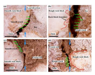
**Figure 14.** The characteristics of cracks at the soil–rock interface and ice–rock interface: (a) smooth ice–rock interface crack; (b) rough ice–rock interface crack; (c) smooth soil–rock interface crack; (d) rough soil–rock interface crack.
