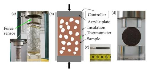
**Figure 3.** The testing apparatus and method: (a) uniaxial compression test; (b) sketch of the testing system; (c) thermometer probe; (d) Brazilian test.
