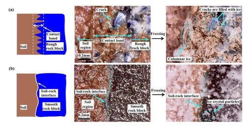
**Figure 11.** The morphology of soil–rock interface (contact band) before and after freezing: (a) rough soil–rock interface (contact band); (b) smooth soil–rock interface.
