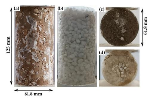
**Figure 2.** Fabricated samples: (a) cylindrical frozen soil–rock mixture sample; (b) cylindrical ice–rock mixture sample for compression testing; (c) disk soil–rock mixture samples for Brazilian testing; (d) disk ice–rock mixture sample for Brazilian testing.
