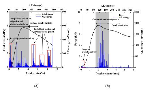
Figure 7. AE characteristics of FSRMs: (a) uniaxial compression test; (b) Brazilian test.
