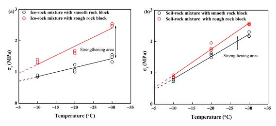
Figure 13. Relationship between indirect tension strength and frozen temperature (a) ice–rock mixture; (b) soil–rock mixture.
