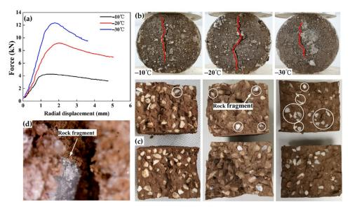
**Figure 6.** Failure patterns of FSRMs under Brazilian testing: (a) radial force–displacement curves; (b) failure patterns; (c) the rock fragments in the tensile cracks; (d) fracture morphology of a rock fragment.
