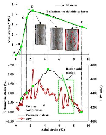
Figure 9. Stress–strain–UPV diagrams showing the different compression stages.
