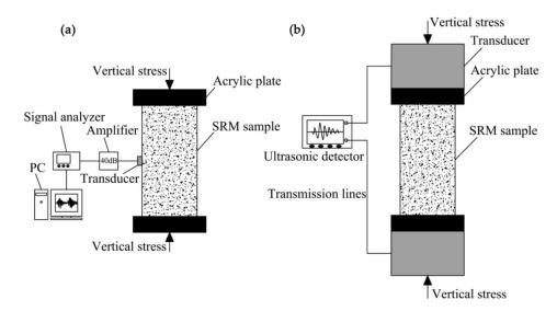
Figure 4. Testing system: (a) acoustic emission (AE) system; (b) ultrasonic plus velocity (UPV) system.
