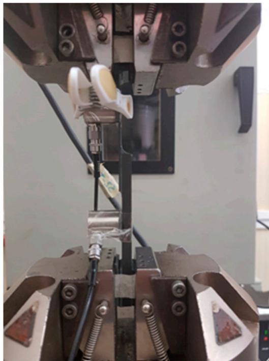
**Figure 2.** Experimental setup with AE sensors mounted on the specimen.
