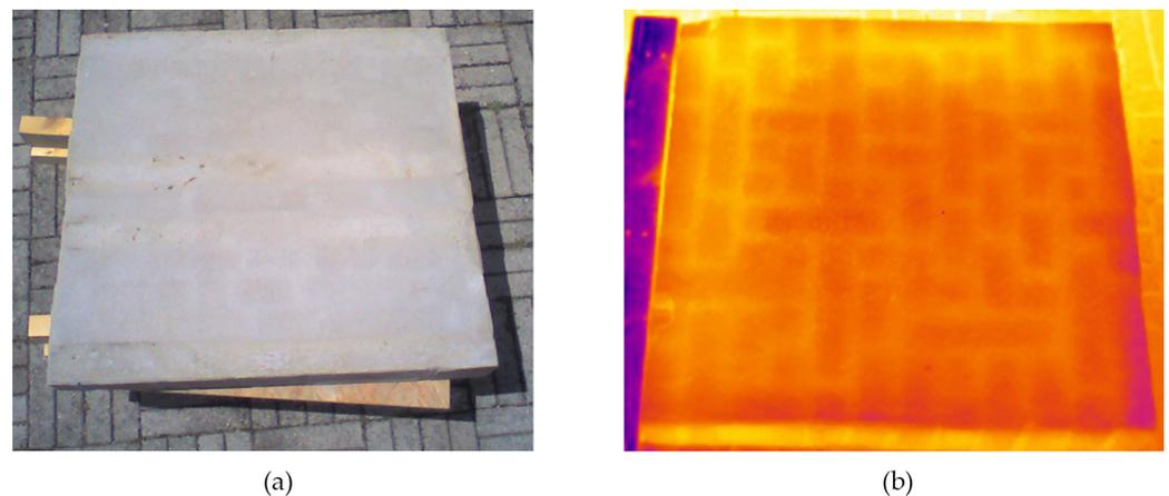
**Figure 5.** Preliminary tests of thermographic imaging. (a) Quasi-periodic masonry wall sample covered with plaster. (b) Its thermographic image.
