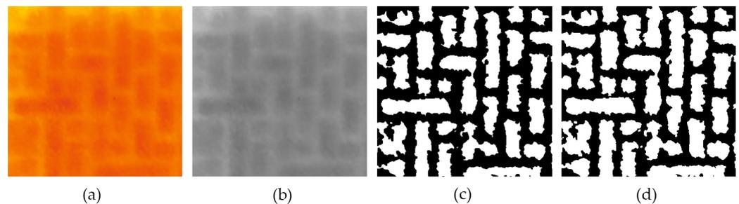
**Figure 7.** Identified texture of random masonry sample: (a) thermographic image, (b) surface temperature as greyscale values  $T_i(x, y)$ , (c) black and white image after thresholding  $b_i(x, y)$ , (d) identified texture after erosion and dilation,  $b_d(x, y)$ .
