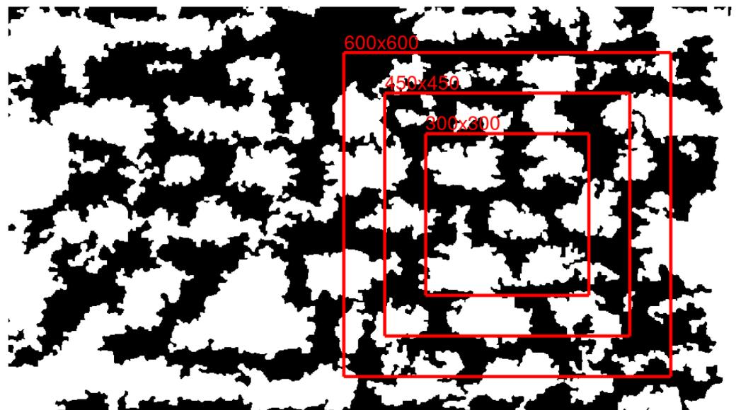
Figure 14. Test-windows used for the estimation of elastic characteristics of the masonry texture.
