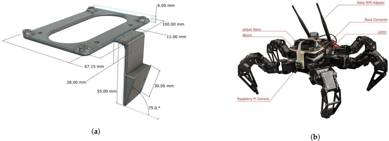
**Figure 3.** Hexapod physical augmentations and peripherals (a) CAD rendering of physical mounts for peripherals (b) modified PhantomX platform with Jetson Nano controller, Raspberry Pi Camera V2, buck converter, U2D2, and Netis AC wireless adapter.
