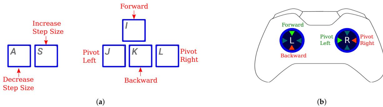
**Figure 9.** Evaluated operator interfaces to be compared against the proposed haptic interface **H** (a) keyboard layout for operator interface **K** (b) game controller mapping for operator interface **J**.
