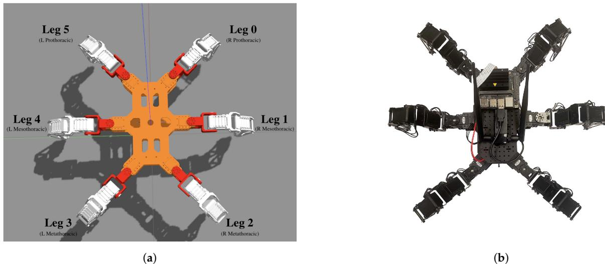
**Figure 1.** Trossen Robotics PhantomX hexapod (a) leg enumeration, rendered and simulated in ROS Gazebo (b) physical implementation of hexapod robot. For alternating tripod gaits odd enumerated legs move separately from even legs.
