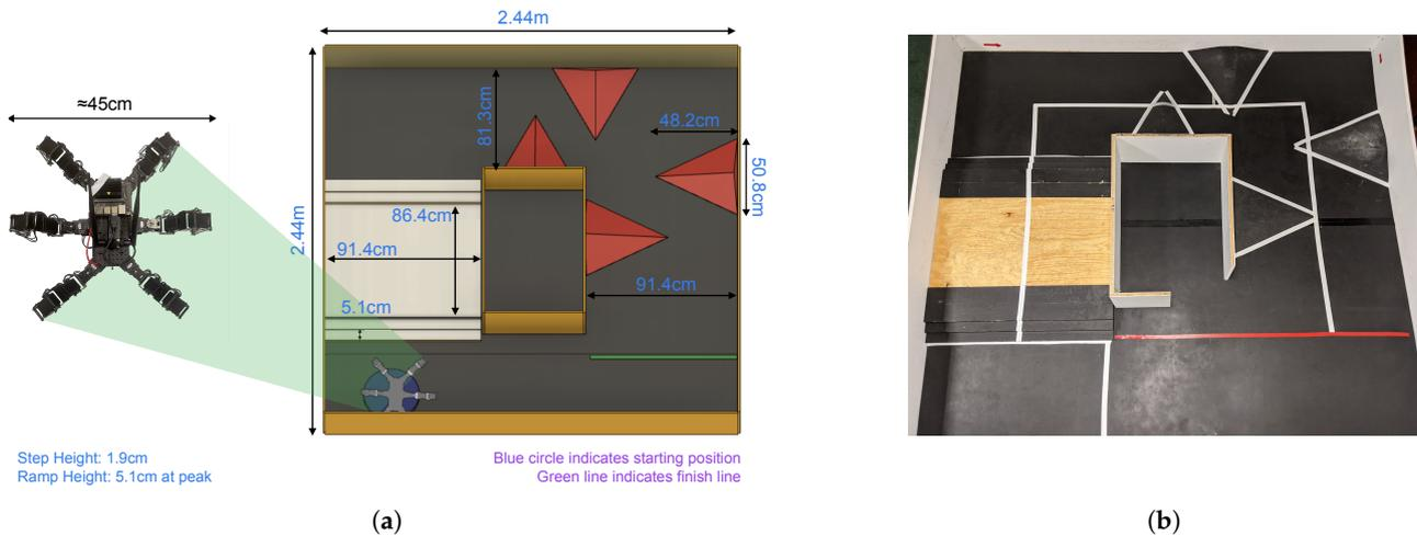
**Figure 10.** Obstacle course for Experiment II (a) CAD rendering with dimensions and (b) physical realization. The goal is to start from the bottom left corner and navigate clockwise to the bottom right.
