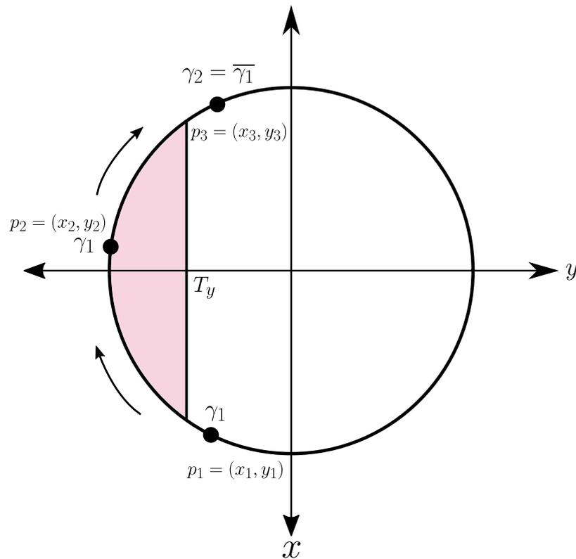
**Figure 6.** Pivoting phase is determined solely by transitions from outside to within the shaded region, determined by  $T_y$ . As the commanded position coordinates shift from  $p_1$  to  $p_2$ , the cursor enters the shaded region and the  $y$  position is less than  $T_y$ . When the cursor next leaves the shaded region, for example to  $p_3$ , the phases of the rotation is toggled, which alternates which set of three legs are raised.
