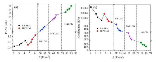
**Figure 8.** The effect of energy density E on the (**a**) PCAS and the (**b**) cooling rate of the as-forming AISI 316 L stainless steel samples at different processing parameters by LPBF and DED [49].
