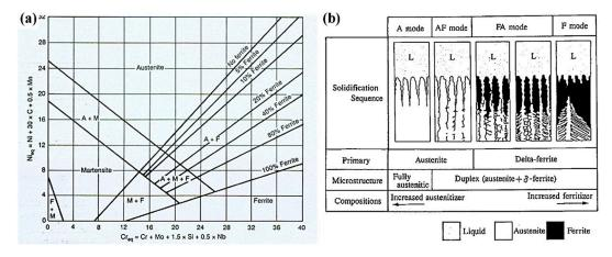
Figure 9. (a) Schaeffler's diagram and (b) austenitic steel solidification diagram [41].
