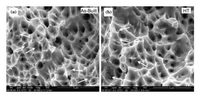
**Figure 15.** Fracture surfaces of AISI 316L stainless steel: (a) as-built and (b) heat-treated. Arrows mark a few of the many examples of fine particles observed resting inside ductile dimples throughout the fracture surface [90].
