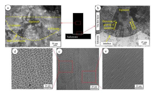
**Figure 4.** Light optical microscopy micrographs of the DED AISI 316L steel samples produced by DED: (a) a representative melt pool at the middle height, (b) the microstructure of the first layer, (c) SEM images of the columnar and equiaxed microstructures referring to the last deposited layer, (d,e) high magnifications of (c) from two different regions [37].
