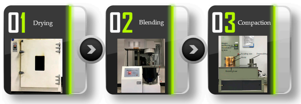
Figure 2. Preparation procedure of AC-13 by the superpave gyratory compaction (SGC) method.
