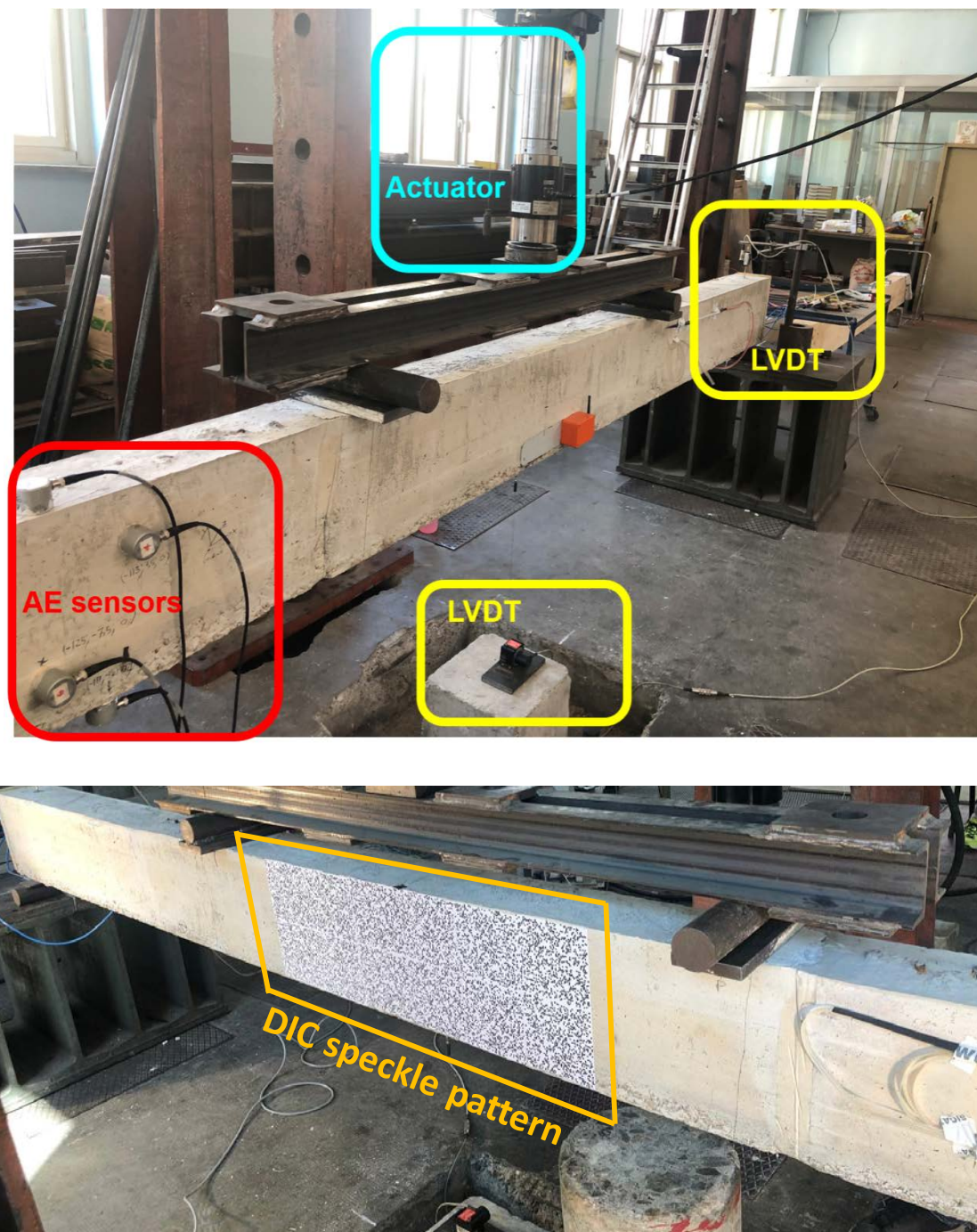
Figure 2. Front ( top ) and back ( bottom ) sides of the test setup showing the servo hydraulic actuator, the linear variable differential transformer (LVDT) sensors, the location of some AE sensors, and the speckle pattern on the central beam surface for digital image correlation (DIC) applications.
