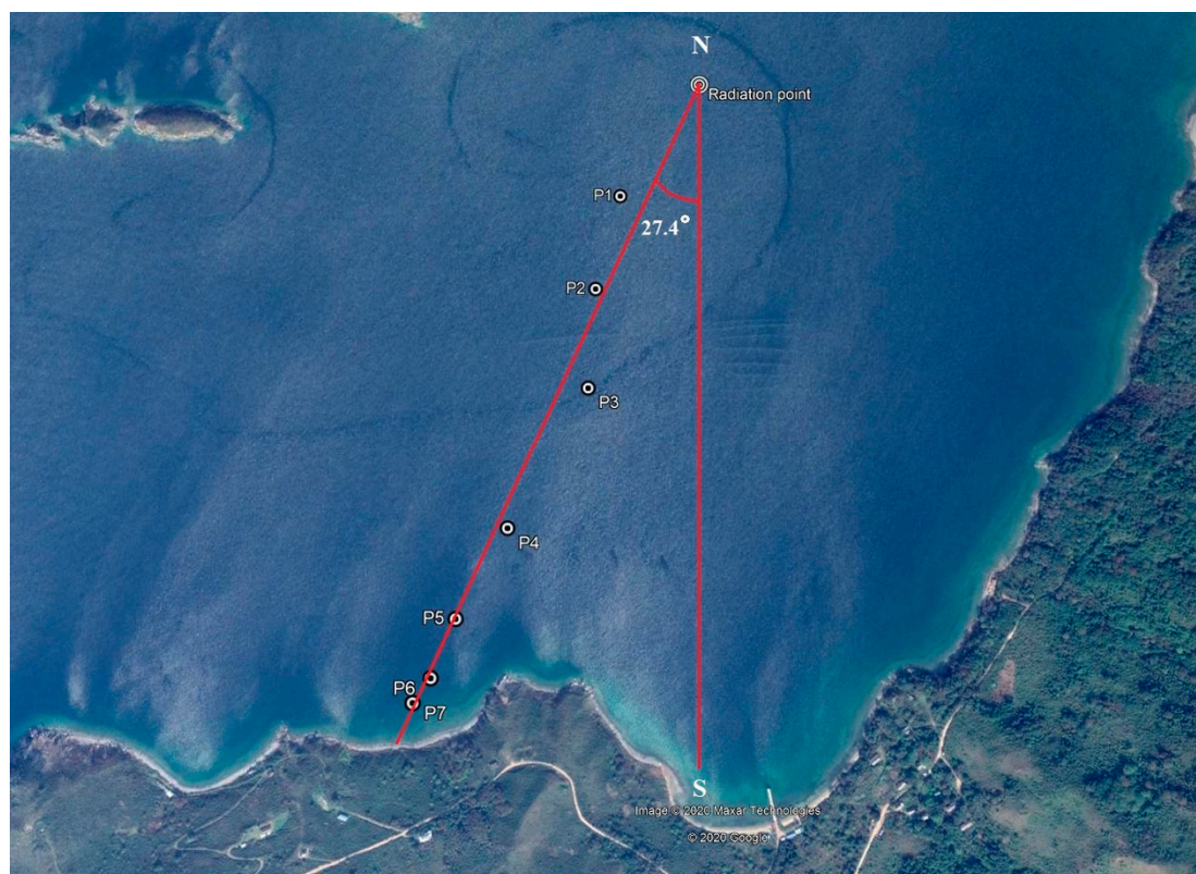
Figure 1. Map scheme of the experiment. The labelled “radiation point” is the location of the vessel with the transmitter. Points P1–P7 show the positions of the receiving stations. The angle 27.4° is the angle between the reception route and the “North–South” direction.
