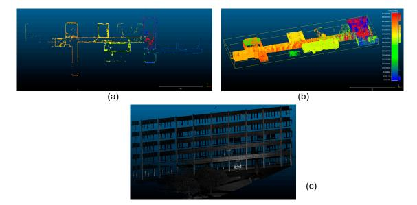
Figure 14. Samples of Zeb point cloud data (a,b) and terrestrial point cloud data (c).
