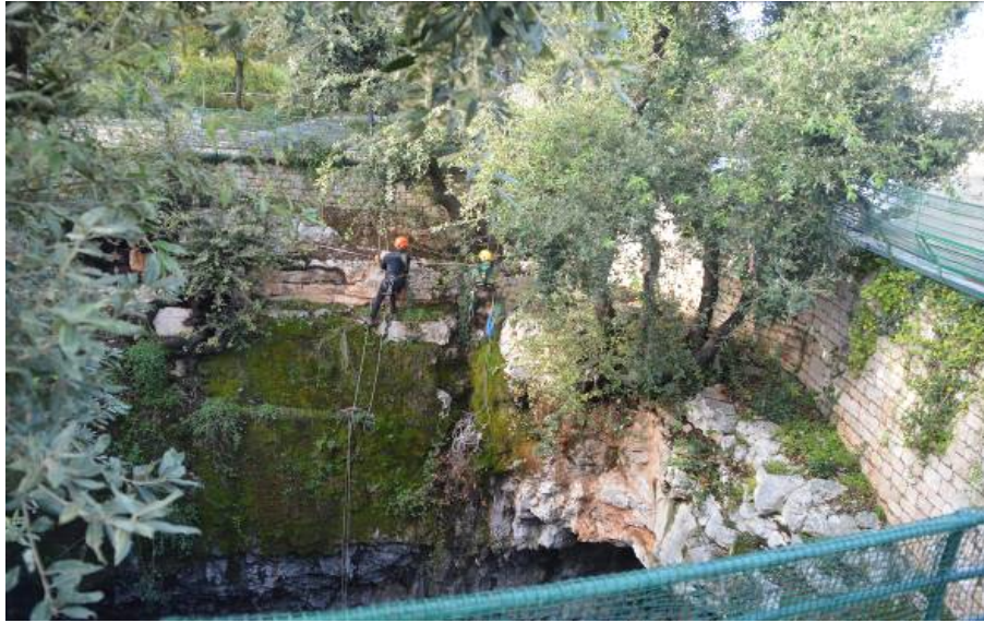
Figure 14. Acquisition phase of geo-mechanical data with standardized techniques (scanline by geologist rock climbers).
