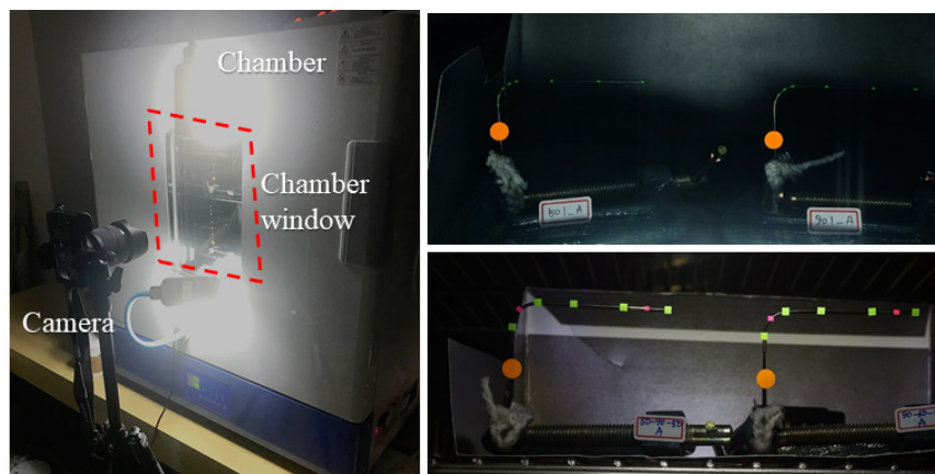
Figure 5. Test and measurement set-up and specimens in chamber.
