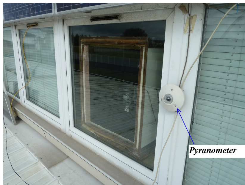
Figure 3. Pyranometer used to measure the global vertical solar radiation.
