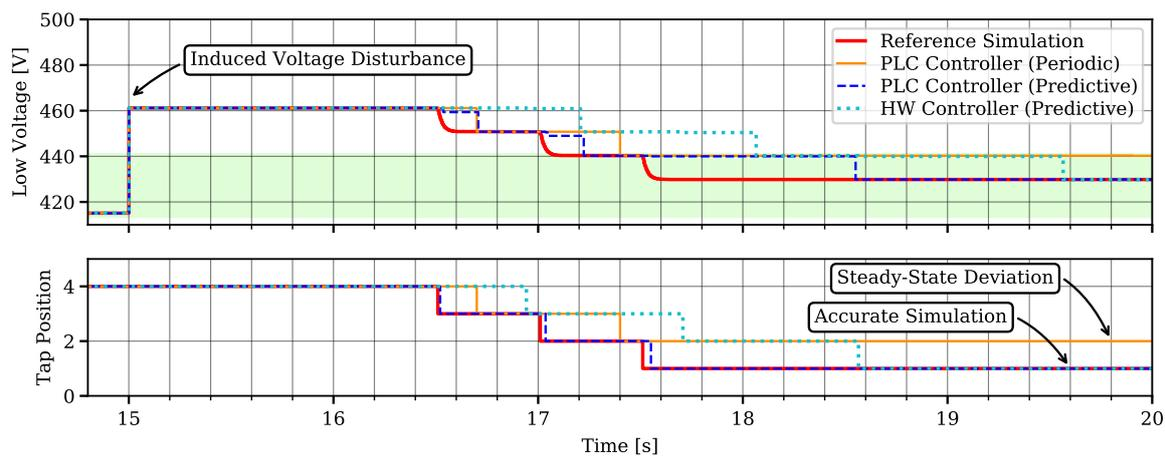
Figure 5. Exemplary switching operation.
