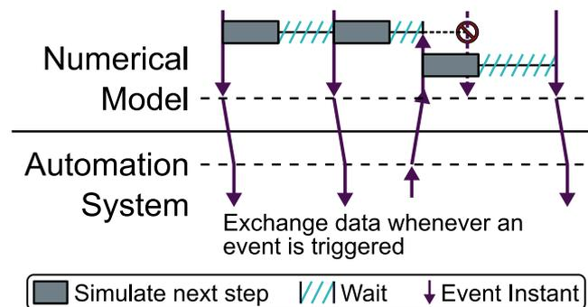
**Figure 3.** Predictive event mapping: Predicted events will be invalidated and updated as soon as events from the automation system arrive.
