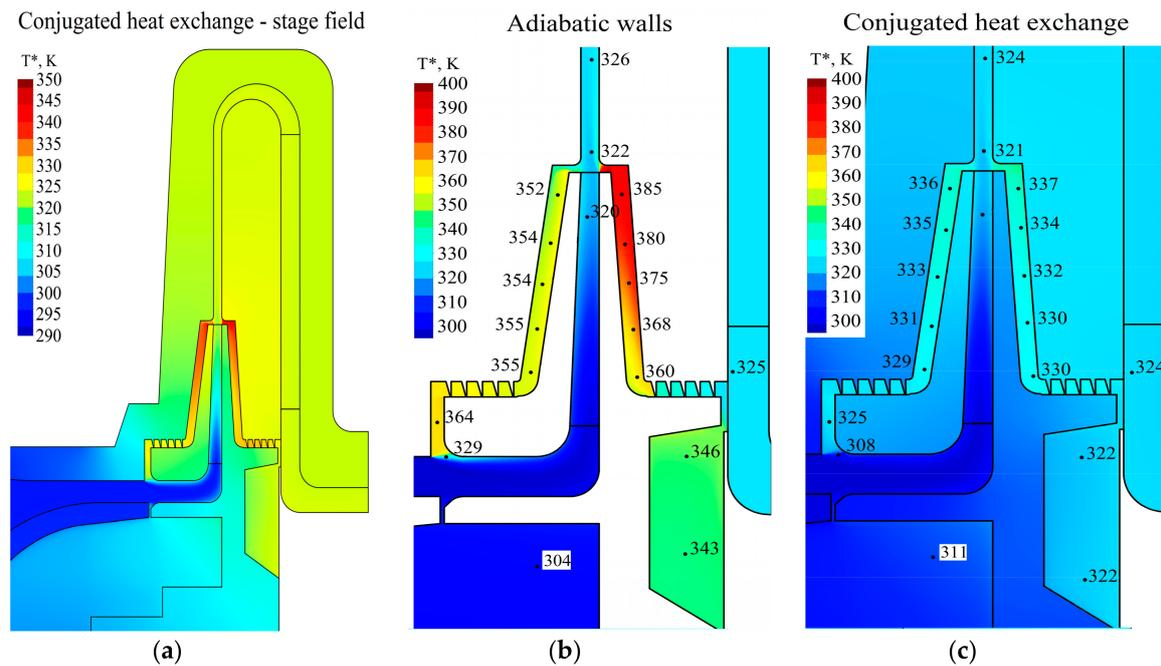
**Figure 3.** Full temperature field. (a) In optimal mode for the model with a conjugate heat exchange of the flow part; (b,c) For the model with adiabatic walls and a conjugate heat exchange, respectively.
