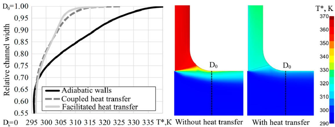
Figure 4. Temperature profiles at the inlet to the impeller for three variants of flow part heat exchange.
