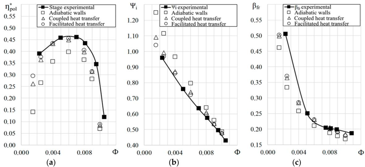
Figure 2. Gas-dynamic characteristics of the SVD-1 stage, taking into consideration the surfaces' heat exchange as compared with the experimental data. (a) Polytropic efficiency  $\eta^*_p$  (b) Internal pressure coefficient  $\psi_i$  (c) Disk friction coefficient  $\beta_{fr}$ .
