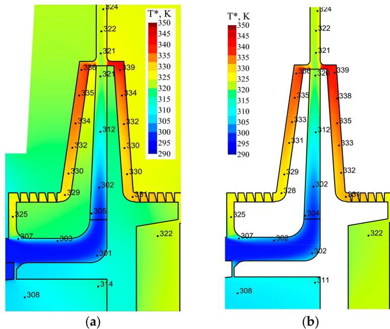
**Figure 7.** The comparison of temperature fields. (a) In the impeller with the conjugate heat exchange; (b) In the simplified accounting method of the heat sink.
