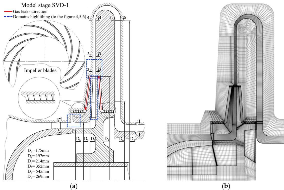
**Figure 1.** (a) Sketch of the model stage SVD-1 flow part and leakage diagram (red arrows); (b) The SVD-1 stage mesh model for conjugate heat transfer modeling.
