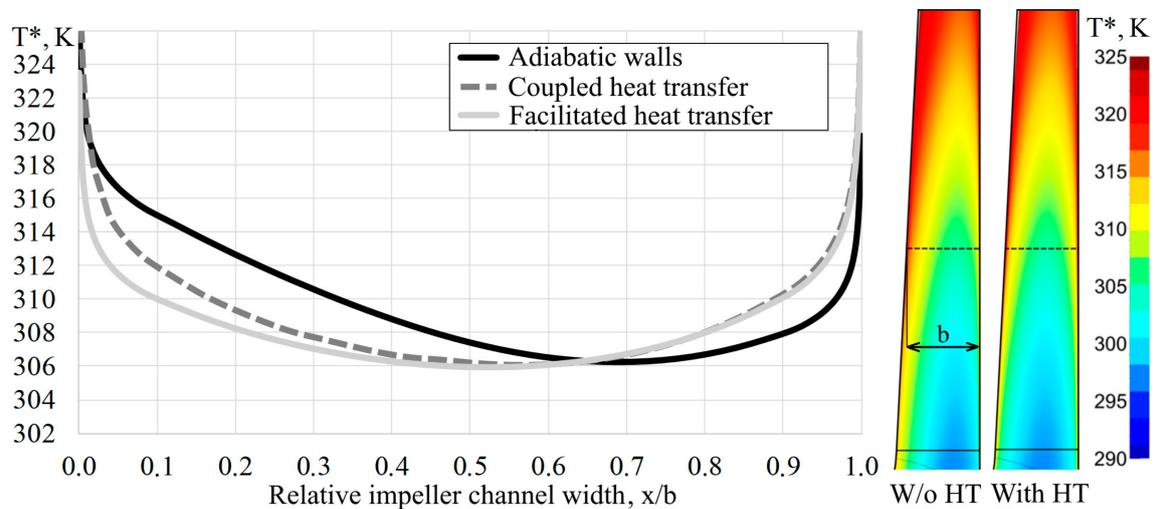
Figure 5. Temperature profiles in the average cross-section of the impeller blade in diameter for three variants of flow part heat exchange.
