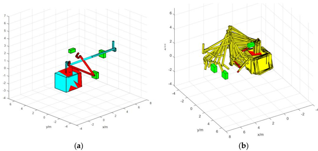
**Figure 4.** Initial configuration, final configuration, and movement history of the space robot in Scenario 1. (a) The final configuration solved by the planning algorithm in Scenario 1; (b) The movement history of the space robot from the initial configuration to the goal EE position in Scenario 1.
