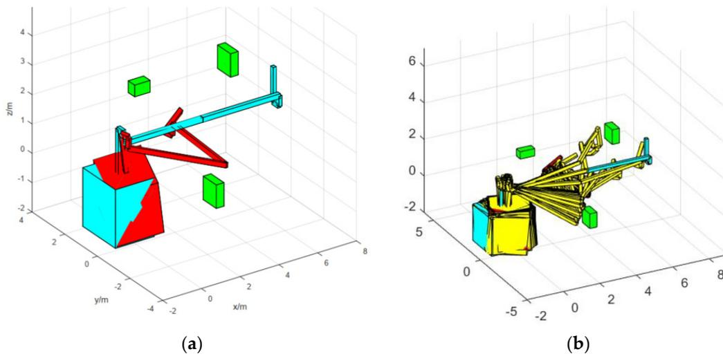
**Figure 6.** Initial configuration, final configuration, and movement history of the space robot in Scenario 2. (a) The initial configuration and the final configuration solved by the planning algorithm in Scenario 2; (b) the movement history of the space robot from the initial configuration to the goal EE pose in Scenario 2.
