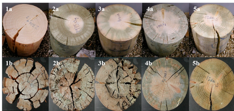
Figure 3. Effect of brown rot fungi on wood pole segments before (1a–5a) and after 24 months incubation (1b–5b). 1; Control. 2; copper-chromium (CC) treated poles. 3; (Bis-(N-cyclohexyldiazeniumdioxy)-copper) (Cu-HDO) treated poles. 4; copper-chromium-boron (CCB) treated poles. 5; Alkaline Copper Quaternary (ACQ) treated poles.
