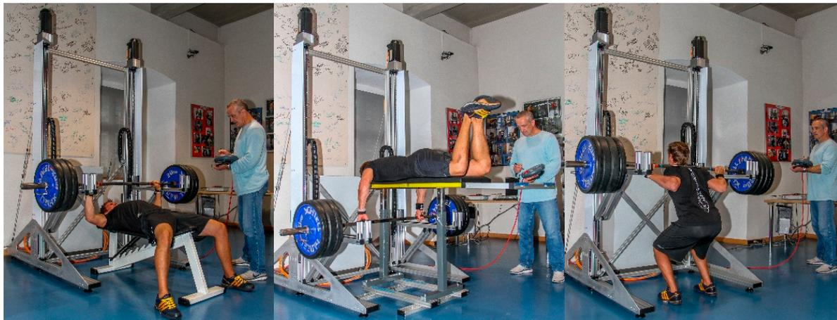
**Figure 1.** The Intelligent Motion Lifter© (IML) prototype in 2010. From left to right: bench press, bench pull and squat.
