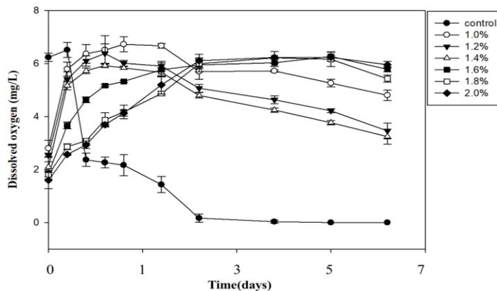
Figure 4. Effect of alginate concentration on the release profile of dissolved oxygen.
