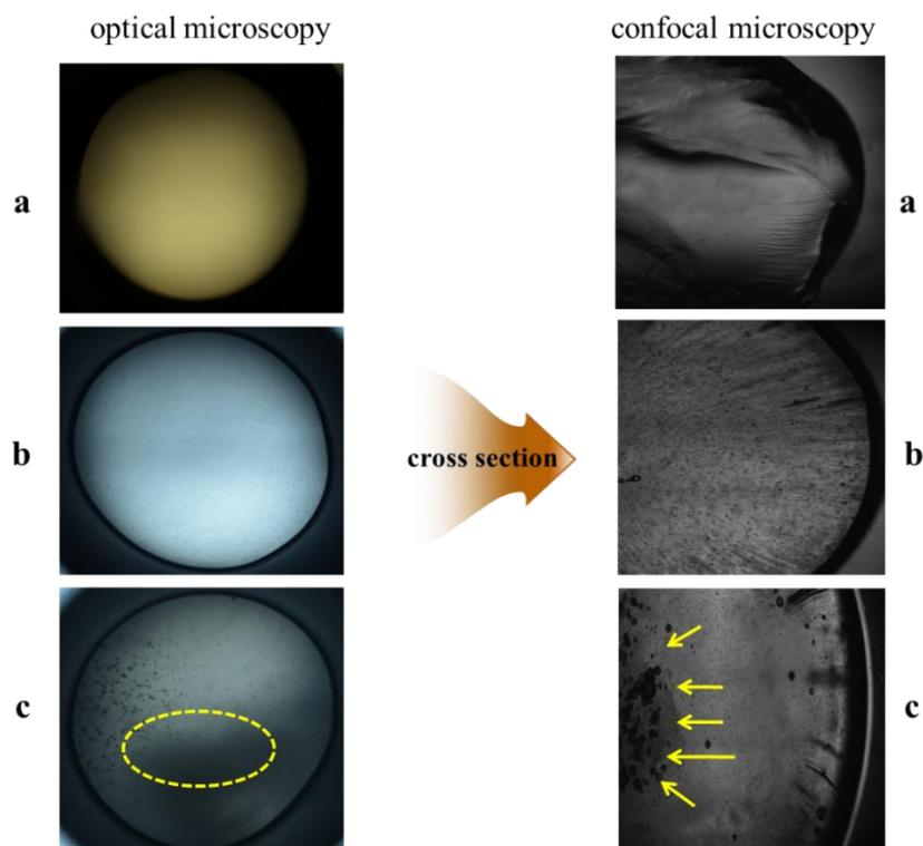
**Figure 3.** Capsule morphology observed by optical microscopy (left, ×50), and confocal microscopy (right, ×100): (a) control (b) cells-without Ocs\*, (c) cells with Ocs. \* Ocs: oxygen capsules.
