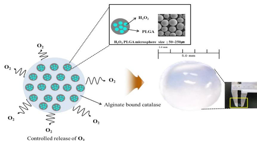
**Figure 1.** Concept of oxygen-releasing system for large-sized tissue regeneration; enhancement of cell and tissue survival by supply of oxygen.
