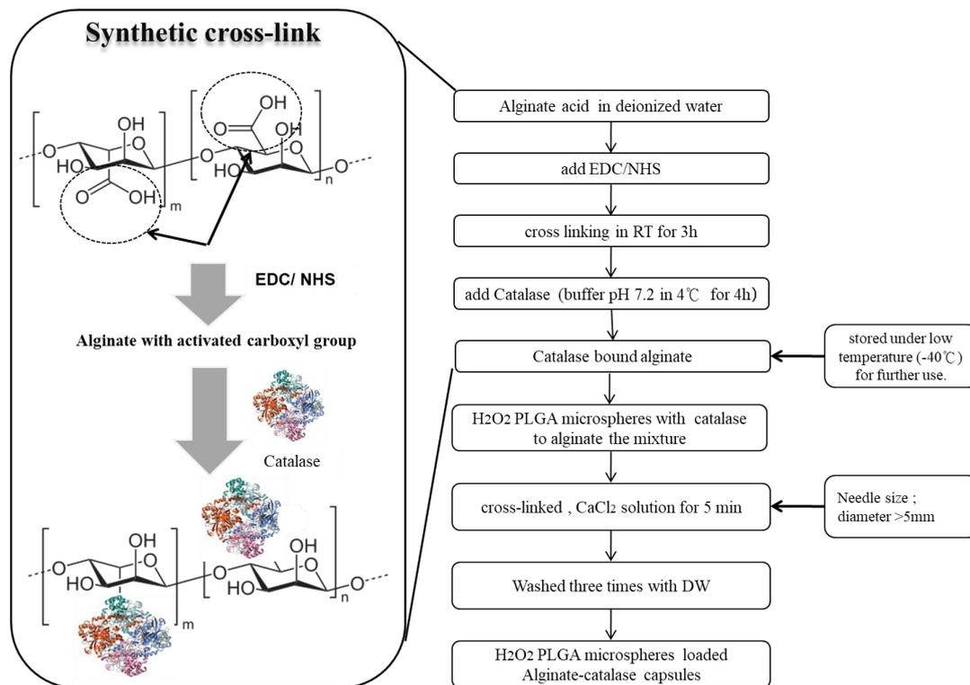
**Figure 2.** Fabrication process of  $\text{H}_2\text{O}_2$  PLGA microspheres loaded alginate-catalase capsules.
