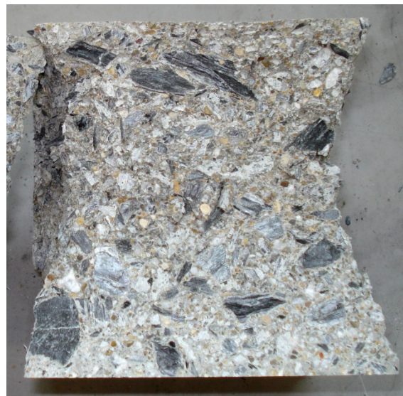
Figure 14. Concrete cube test specimen after compressive strength testing according to Table 7.
