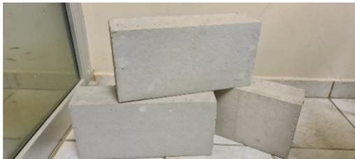
(c) Produced cellular concrete blocks: 0.12 × 0.2 × 0.4 m
