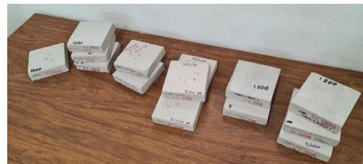
(b) Probes for thermal conductivity, specific heat and density tests: 0.15 × 0.15 × 0.04 m
