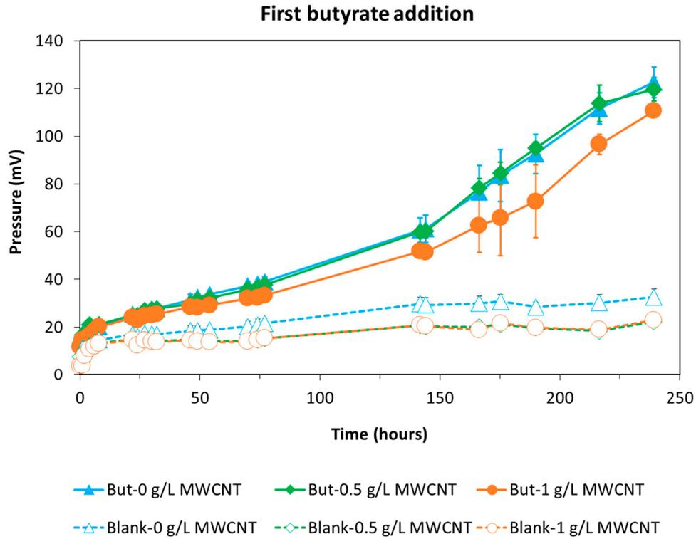
**Figure S3.** Pressure (mV) increase in the assays amended with butyrate (first addition), in the presence of different MWCNT concentrations: 0 g L<sup>-1</sup> ( ), 0.5 g L<sup>-1</sup> (•) and 1.0 g L<sup>-1</sup> (•). Blank assays (no added substrate) are also shown (open symbols). The results presented are the averages and standard deviations for triplicate assays.
