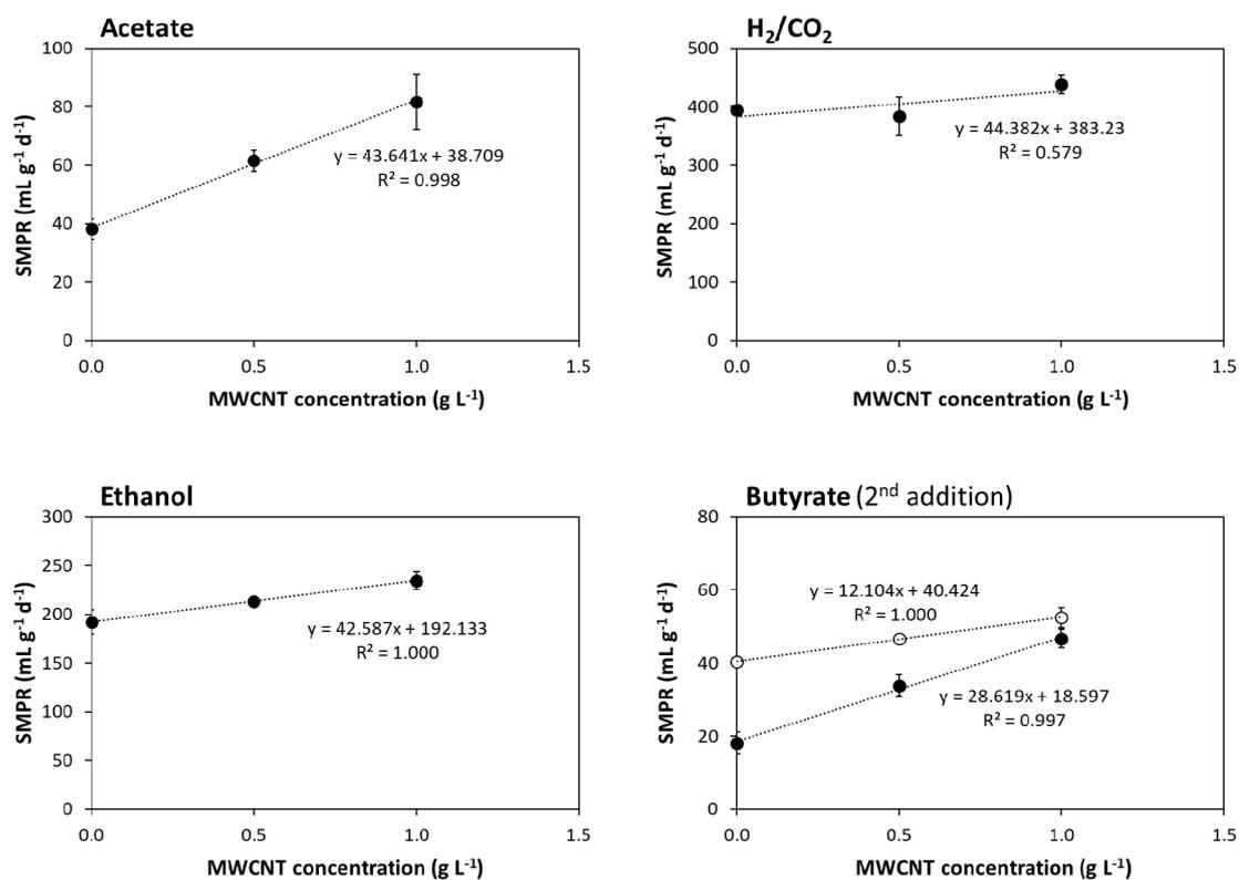
**Figure S2.** Linear correlation between MWCNT concentration and the specific methane production rate (SMPR) for acetate (a), H<sub>2</sub>/CO<sub>2</sub> (b), ethanol (c) and butyrate (2<sup>nd</sup> addition, t = 0-20 h and t > 20 h) (d). Each point is the average of three experimental replicates.
