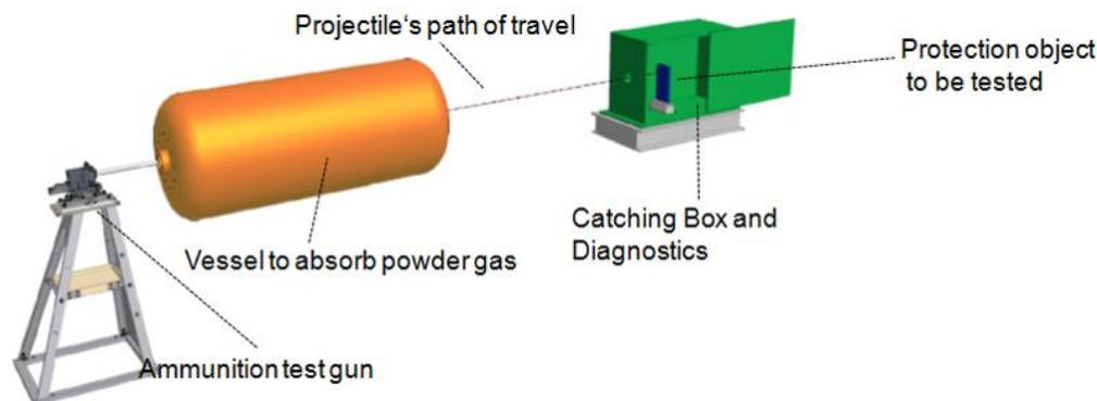
**Figure 1.** Experimental setup for ballistic experiments [16].
