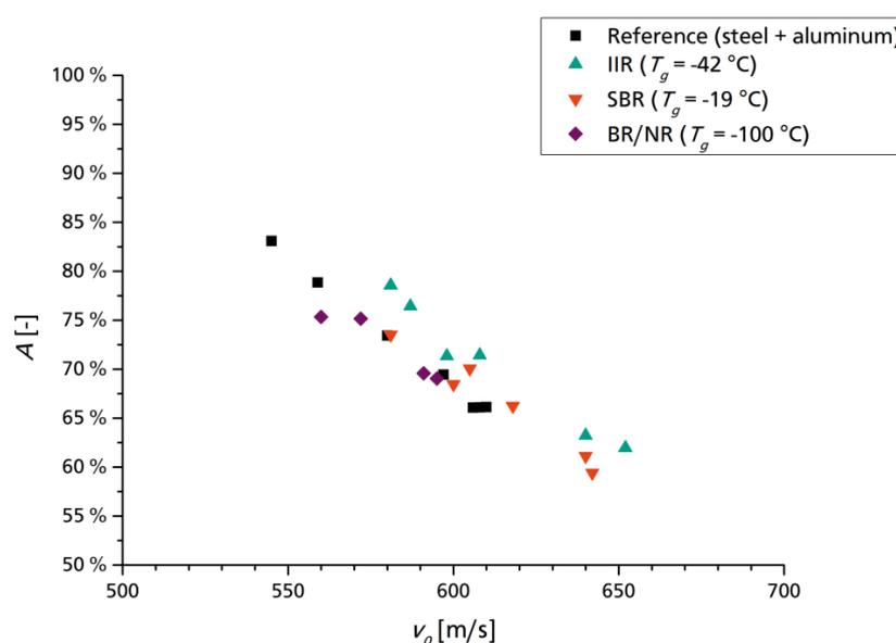
**Figure 9.** Dependency between absorption parameter  $A$  and impact velocity  $v_0$  for different armor configurations.
