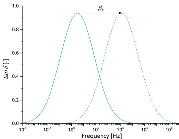
Figure 3. Example of extrapolating a  $\tan \delta$  curve to a different temperature using the shift factor  $\beta_T$ .
