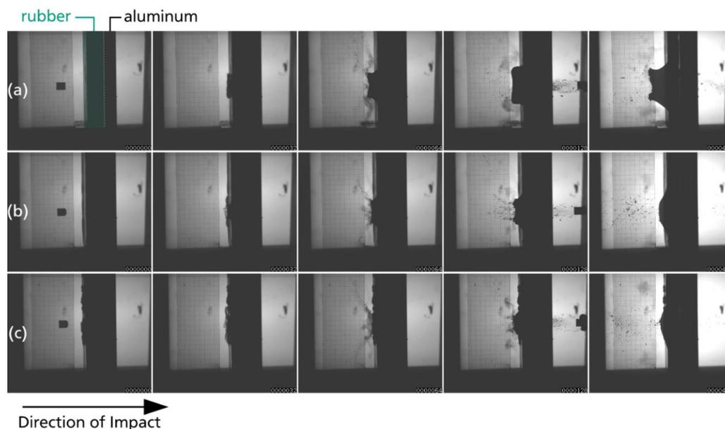
**Figure 8.** High-speed photographs of the impact behavior of (a) BR/NR (9:1), (b) IIR, (c) SBR. Photographs were taken after 0, 32, 64, 128 and 404  $\mu$ s. A schematic colorized overlay in the first photograph (a) highlights the rubber front-layer and aluminum back-layer.
