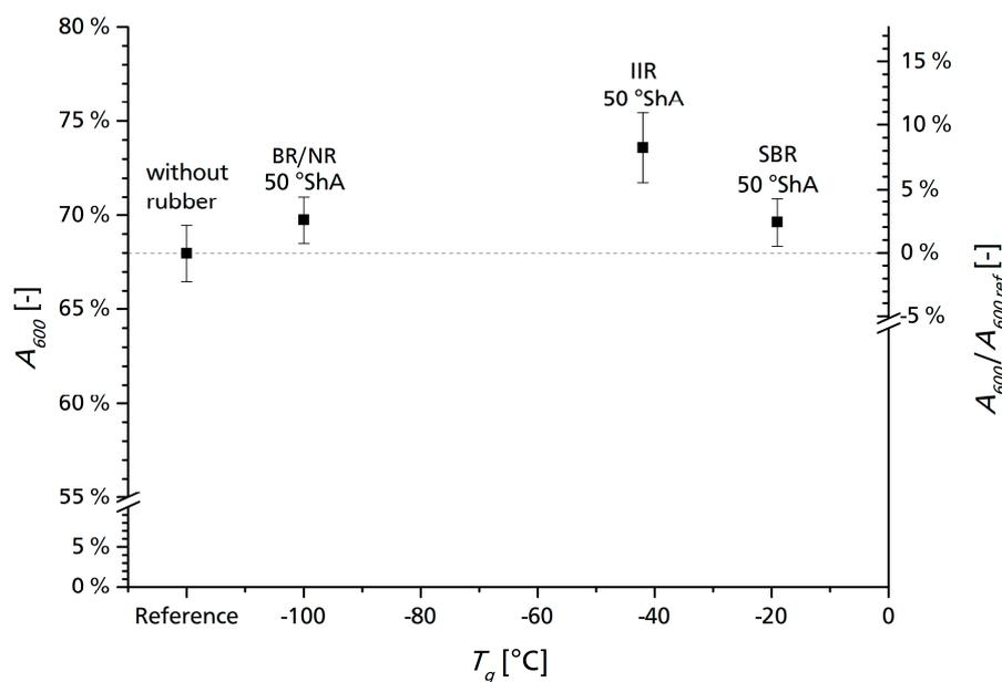
**Figure 10.** Energy absorption during ballistic impact experiments for the configurations with different rubbers. All three rubber compounds possess the same hardness to decrease potential influences besides glass transition and maximized damping.
