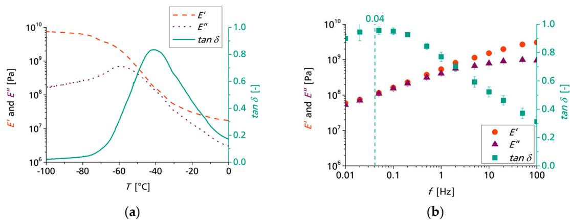
**Figure 5.** (a) Temperature sweep (1 Hz) of butyl rubber from  $-100$  to  $-20$  °C. (b) Frequency sweep of butyl rubber,  $T = -50$  °C. Storage modulus  $E'$ , loss modulus  $E''$  and loss factor  $\tan \delta$  are plotted against temperature (a) and frequency (b).
