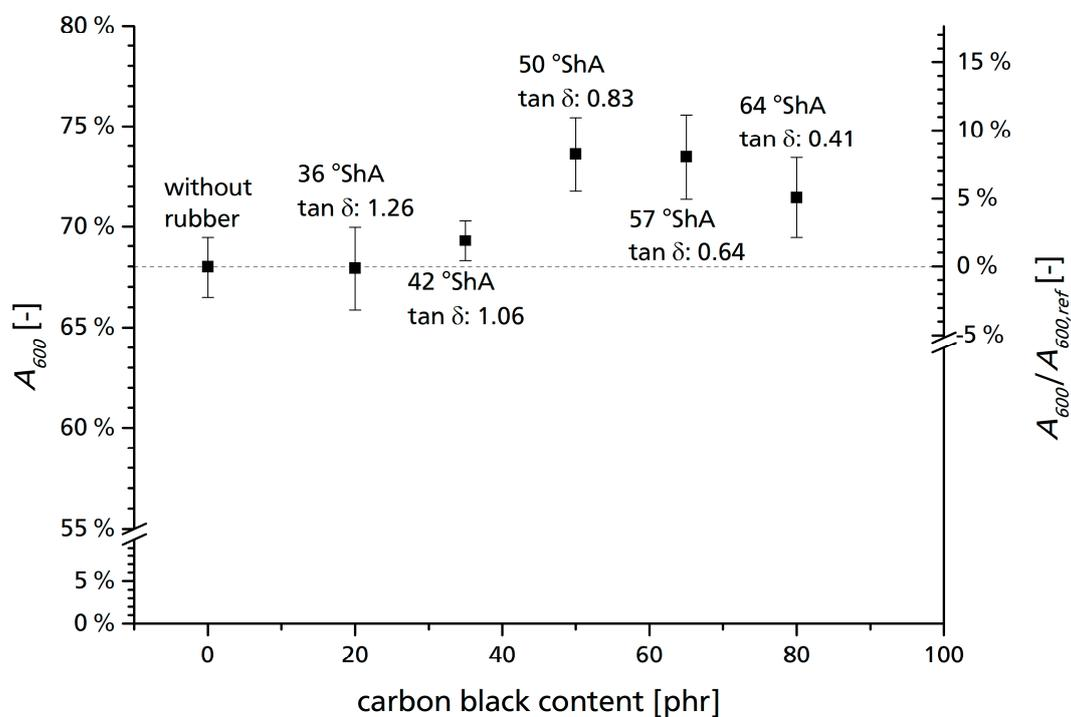
**Figure 11.** Energy absorption during ballistic impact experiments for configurations using IIR formulations with varying carbon black content.
