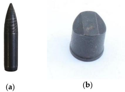
Figure 2. (a) Projectile M352 7.62 × 51 AP. (b) Projectile 7.62 FSP.
