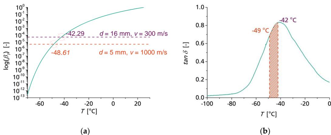
**Figure 7.** (a) Plot of the Williams–Landel–Ferry (WLF) equation with  $T' = 25\text{ }^\circ\text{C}$ ,  $C'_1 = 3.39$  and  $C'_2 = 120.73\text{ K}$ . (b) Temperature sweep of butyl rubber with the corresponding temperature range for impact-induced frequencies.
