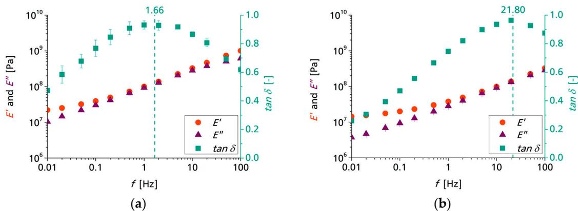
**Figure 6.** Frequency sweeps of butyl rubber: (a)  $T = -40$  °C and (b)  $T = -30$  °C. Storage modulus  $E'$ , loss modulus  $E''$  and loss factor  $\tan \delta$  are plotted against frequency.
