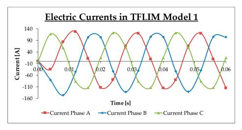
Figure 13. Electric current per phase in model 1.
