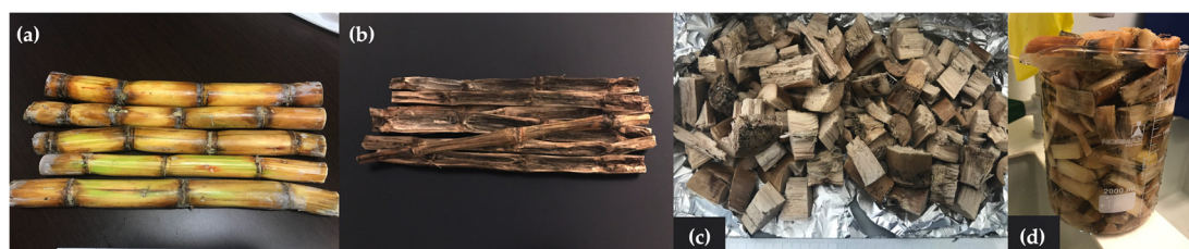
Figure 2. Sequence of procedures to obtain sugarcane pieces used in torrefaction tests: (a) raw material as bought; (b) sugarcane after being processed with the roller mill; (c) sugarcane pieces; and (d) pieces being washed.
