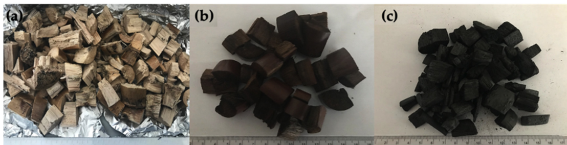
Figure 4. Obtained materials: (a) after drying; (b) after torrefaction at 200 °C; and (c) after torrefaction at 300 °C.
