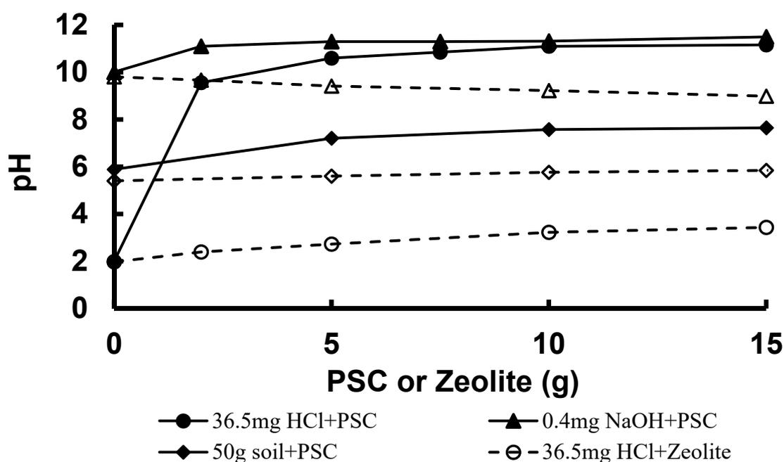
**Figure 1.** Effects of paper sludge carbon (PSC) and zeolite (Z) on the pH of hydrochloric acid, sodium hydroxide, and soil.
