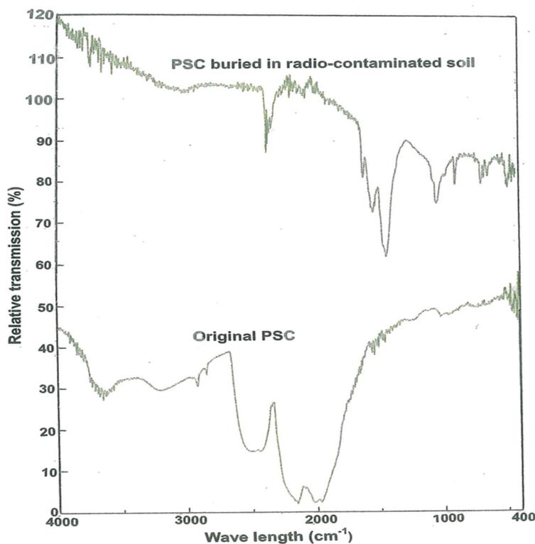
Figure 4. FT-IR spectra of the original PSC and radiocontaminated PSC.
