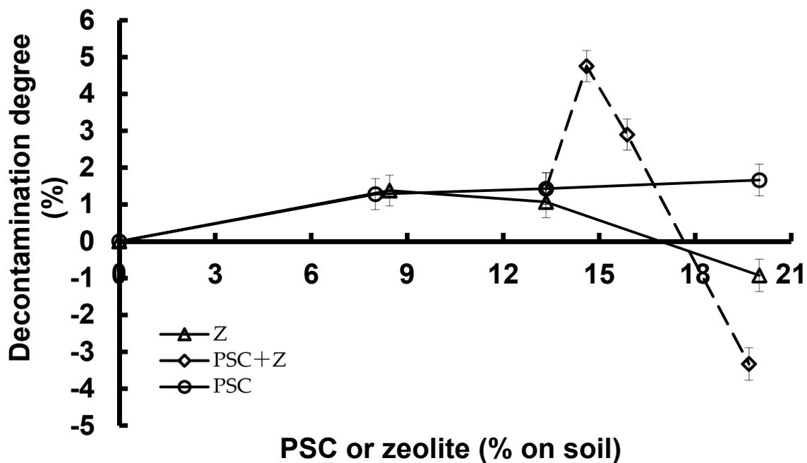
**Figure 2.** Decontamination degrees of the PSC, zeolite (Z), and a combination of PSC and Z.
