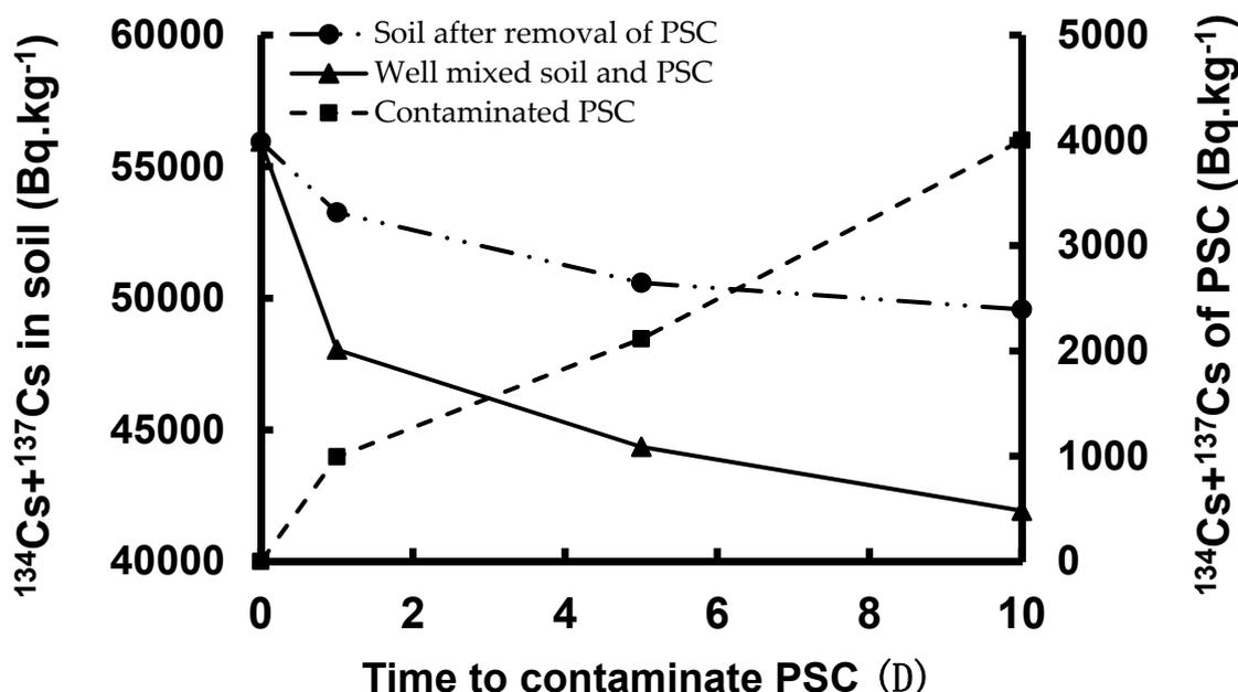
Figure 3. Effect of  $^{134}\text{Cs}$  and  $^{137}\text{Cs}$  in contaminated soil on PSC.
