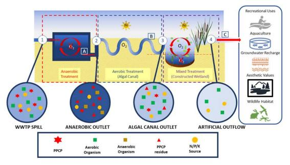
**Figure 6.** Towards the CSCM reactivation, serial system. **A**. Anaerobic bioreactor-pond. Removal of Aerobic microorganisms and PPCPs [229,236]. **B**. Algal canal-contracted wetland. Removal of anaerobic bacteria, PPCPS and PPCPs residue removal [223]. **C**. Mixed treatment (constructed wetland). Remove of nutrients and contaminants. Reuse of zero waste [306].
